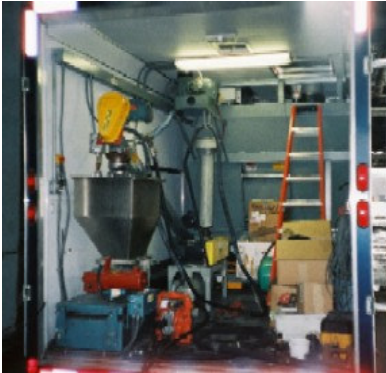
Photograph 6. Sorbent Technologies Sorbent Injection Trailer
