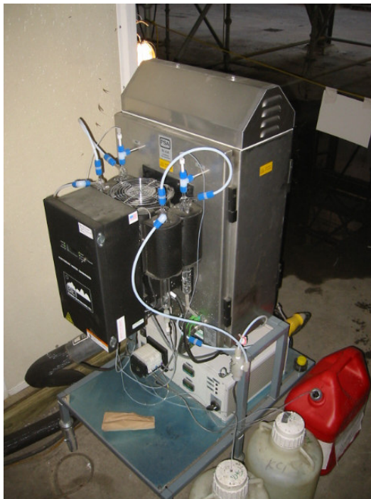
Photograph 7. PS Analytical Wet/Dry Mercury Conversion Module
