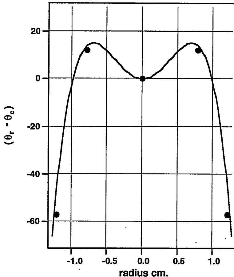
**Figure 7.** Comparison of experimentally measured temperature gradient to model calculations for a 3-D carbon preform
