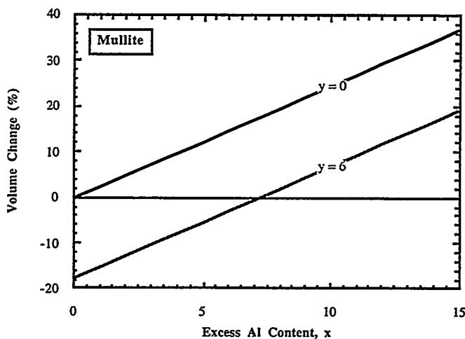
**Figure 5.** The calculated volume change of the mullite preform when reacted with Al to form a ceramic-metal composite. Results are plotted as a function of composite Al content, x, assuming no silicon loss (y = 6) and complete silicon loss (y = 0) following Reaction 3.
