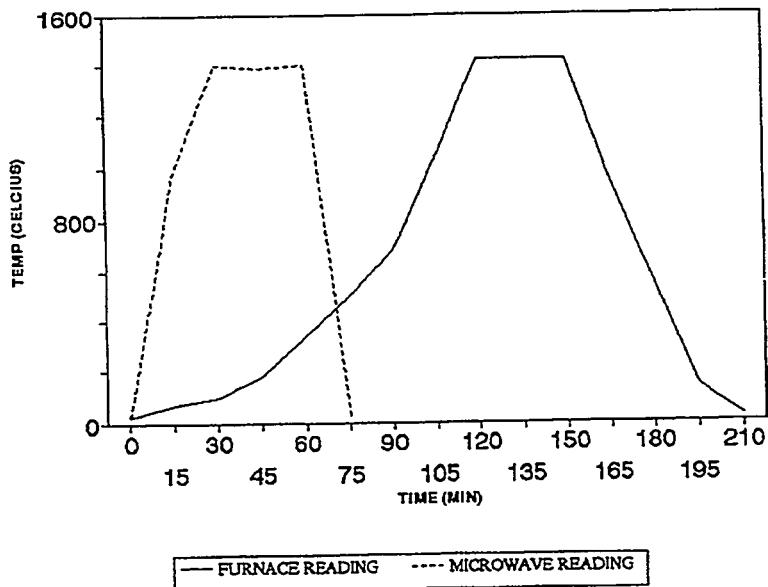
Figure 2: Temperature Profiles for Microwave and Conventional Pyrolysis of PCS
