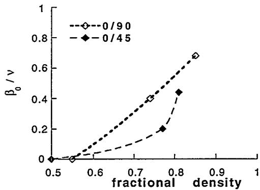
Figure 1: Increase in the number of isolated pores per cubic mm with consolidation for the  $0^\circ/45^\circ$  and  $0^\circ/90^\circ$  weave. Both the number and average size of the pores increases with infiltration.
