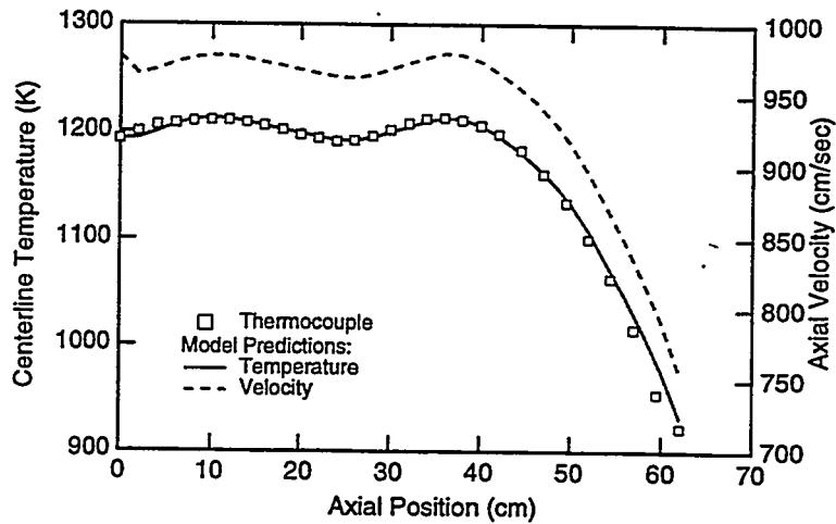
**Figure 5:** CRESLAF prediction of axial velocity in the HTFR based on a fit of the reactor wall temperature axial temperature measurements. Data (squares) correspond to Pt/Rh thermocouple measurements.
