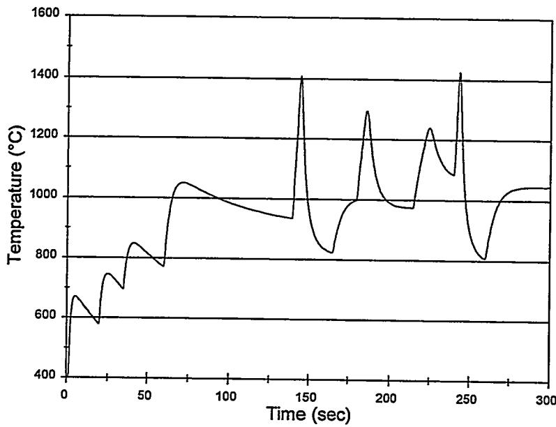
Figure 1b. Numerical simulation of the burst heating observed in a stationary Nextel 550 tow. Step increases in microwave power are indicated by a sudden temperature rise.
