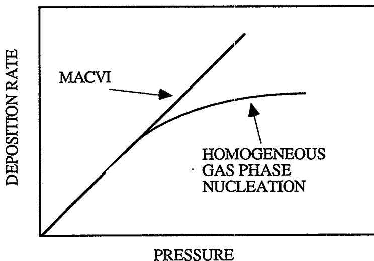
Figure 11. Effect of homogeneous gas phase nucleation on overall deposition rate
