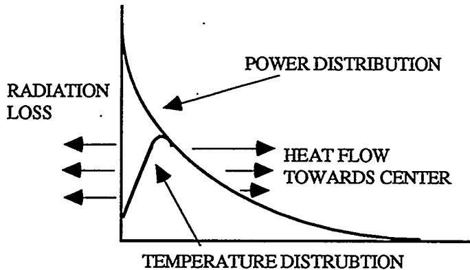
**Figure 1.** The effect of volumetric heating on the temperature distribution.
