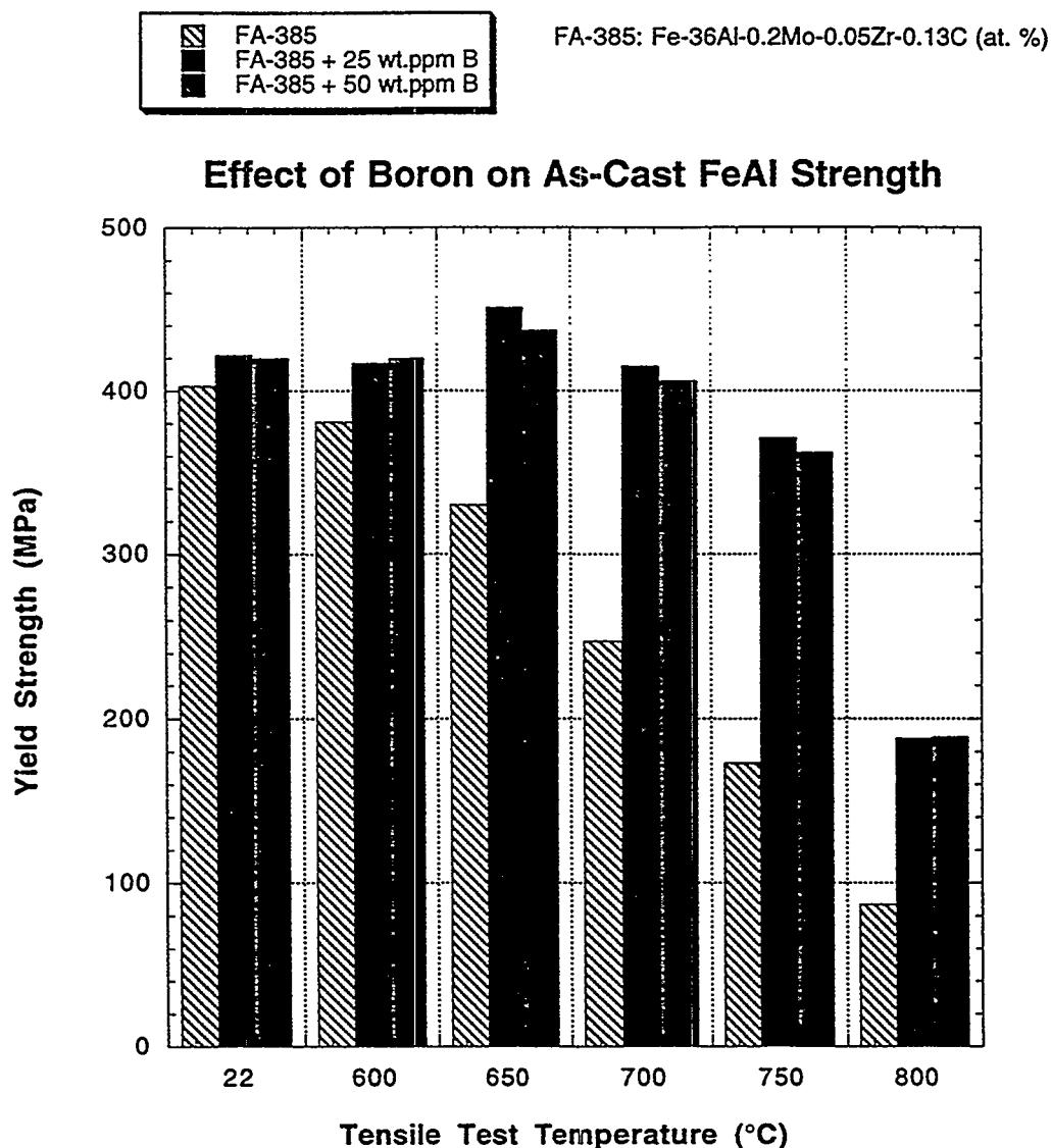
Figure 1 - Yield strength as a function of tensile test temperature for as-cast FeAl alloys (FA-385, -385M1 and -385M2).
