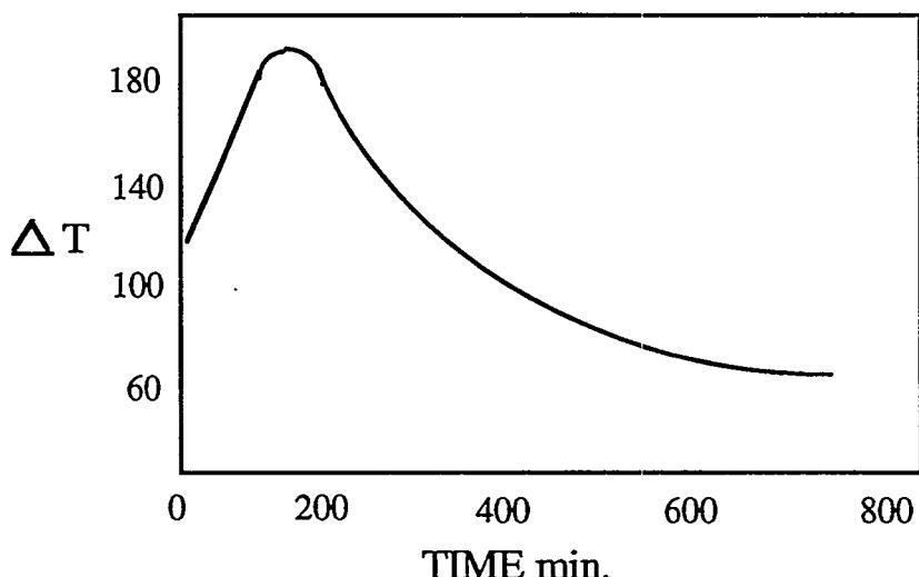
Figure 6. The variation in the temperature gradient as infiltration proceeds.
