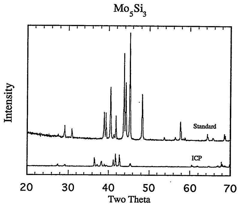
Figure 4. X-ray scan of Mo-Si compound.
