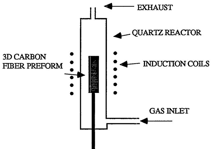
Figure 5. Schematic of the carbon/carbon composite reactor.
