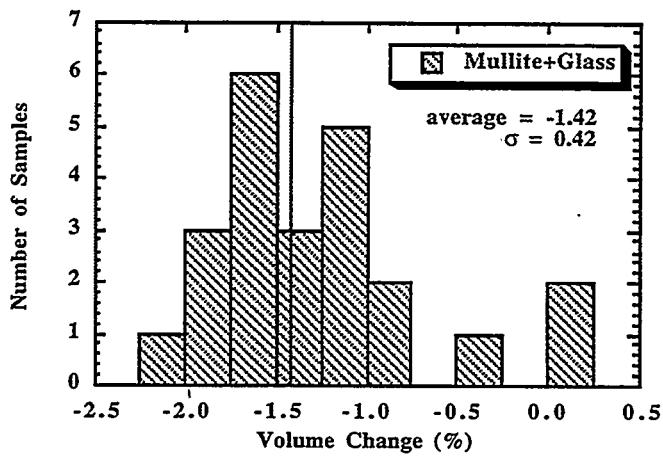
Figure 8. Measured volume changes of 21 different mullite-glass preforms after reaction with Al to form ceramic-metal composites.
