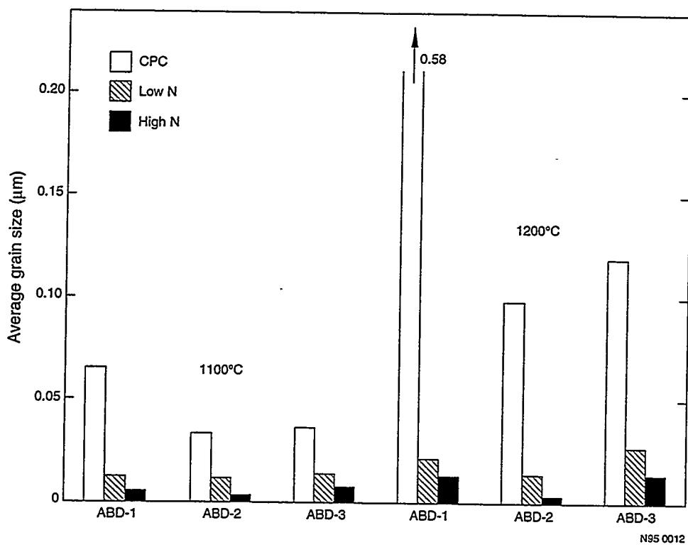
Fig. 2 – Grain sizes after 1 h heat treatments at 1100 and 1200°C for the RSP ABD alloys with high- and low-nitrogen contents, and CPC comparisons.
