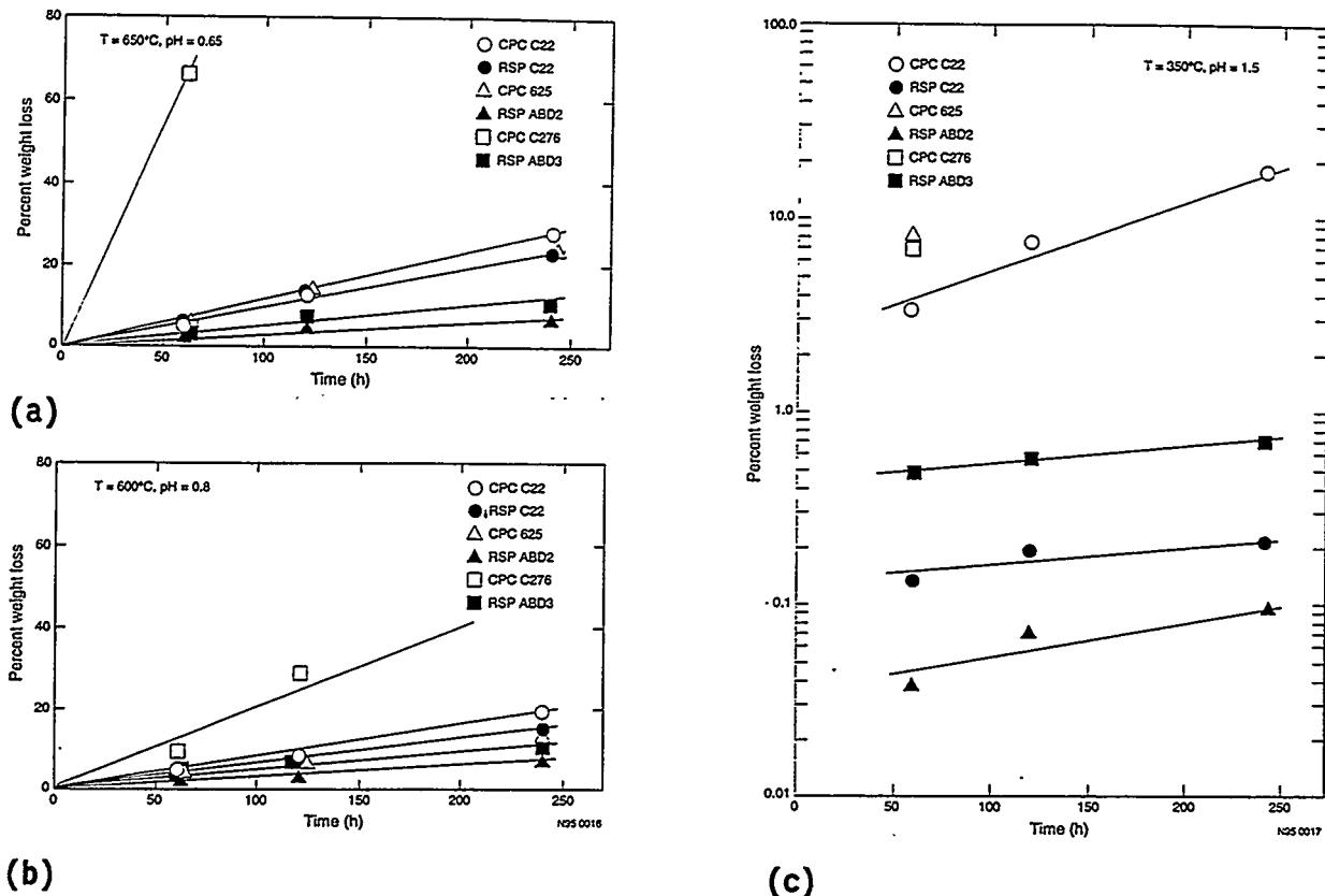
Fig. 5 – Corrosion weight loss of nickel-base alloys for SCWO tests at 240 atm pressure: (a) T = 650°C, pH = 0.65, (b) T = 600°C, pH = 0.8, and (c) T = 350°C, pH = 1.5.
