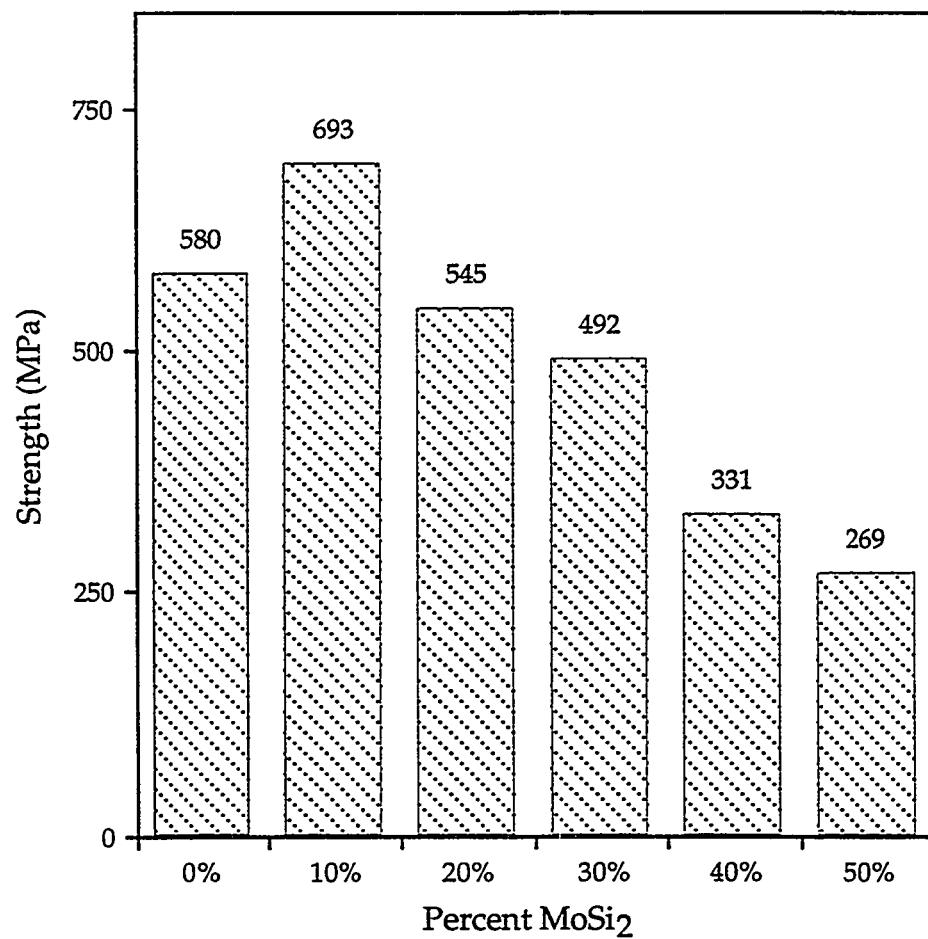
Fig. 17 Four point modulus of rupture for several  $\text{Si}_3\text{N}_4$ - $\text{MoSi}_2$  Composites.
