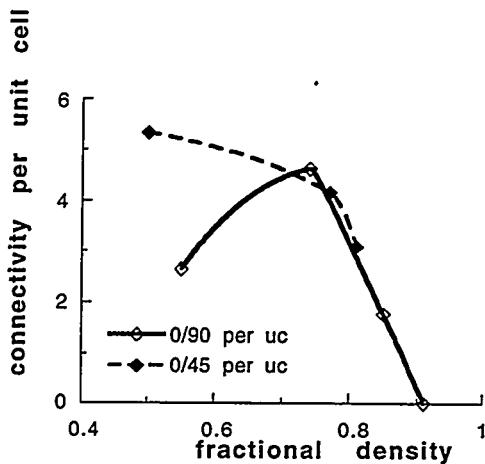
Figure 4: Connectivity per unit cell for both the  $0^\circ/90^\circ$  and the  $0^\circ/45^\circ$  weaves. By about 75% density, the percolating clusters have evolved to topologically equivalent structures in both weaves.
