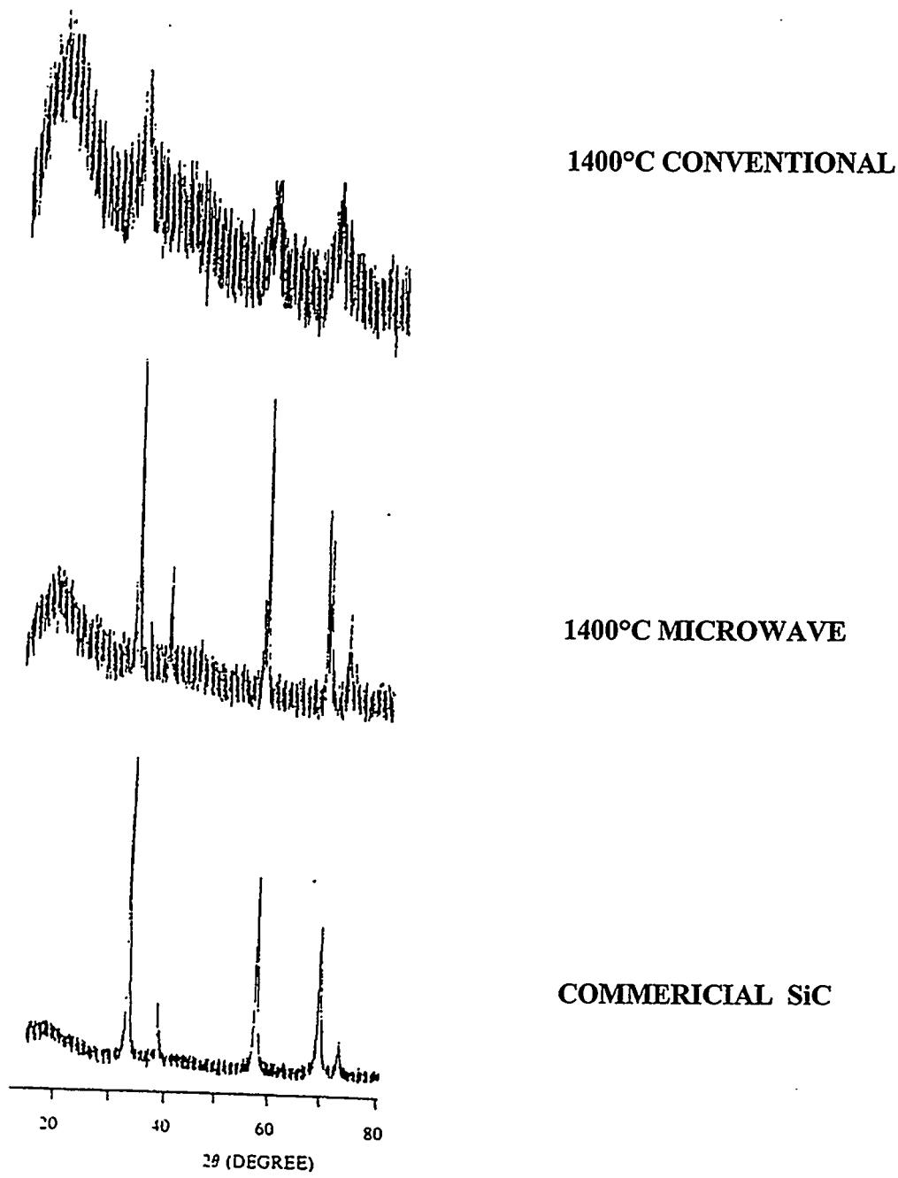
**Figure 3: X-Ray Data for Microwave and Conventional PCS Pyrolysis Product**
