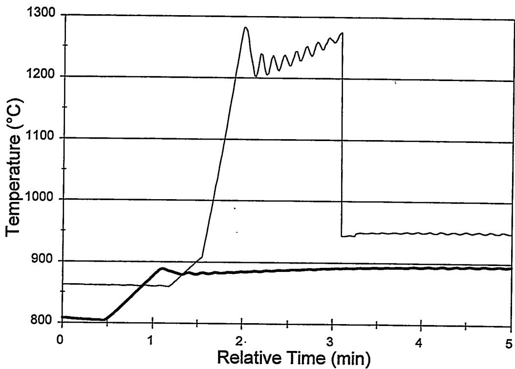
Figure 2. Temperature measurement by the optical fiber thermometer (OFT) in the dual wavelength mode (light line) during heat up from 860°C to 960°C. OFT measured temperature is typically high and remains high until OFT unit is cycled through single wavelength mode back to the dual wavelength mode. Temperature measurement in the single wavelength mode (dark line) is shown for a heatup from 800°C to 900°C.
