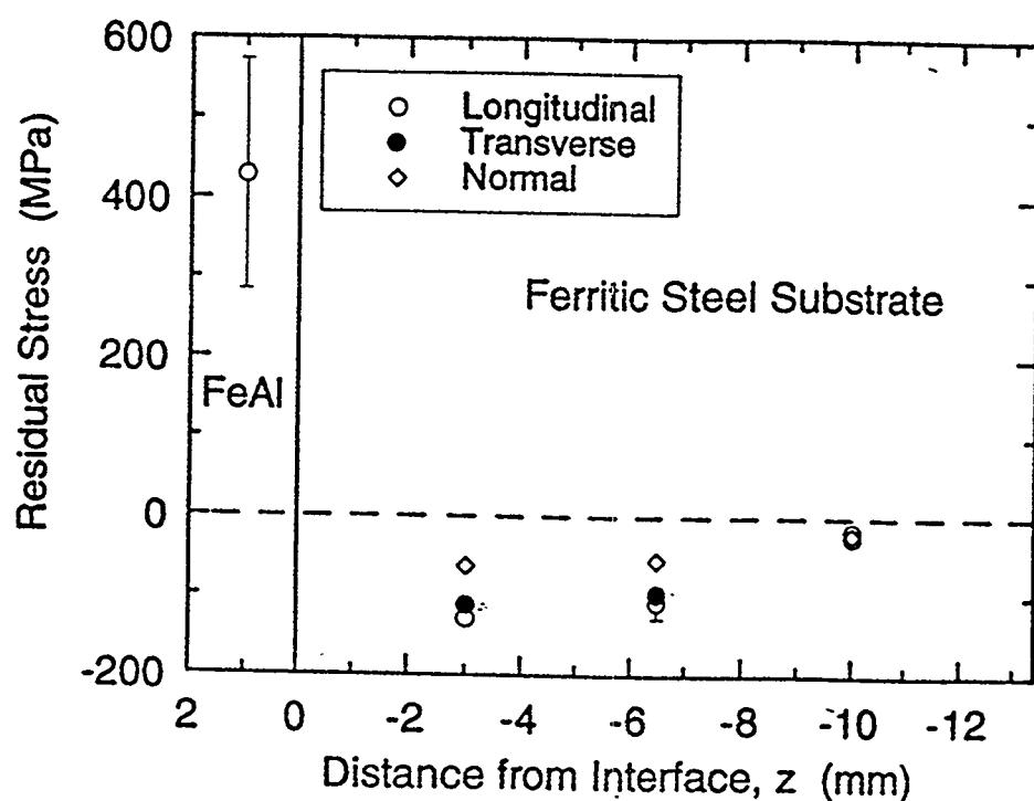
Figure 3. Residual stress in the longitudinal direction as a function of depth in the FeAl weld-overlay cladding and in the 2 1/4 Cr-1 Mo steel substrate. Stresses are calculated from the actual strains measured using neutron-diffraction techniques, as described in-text.
