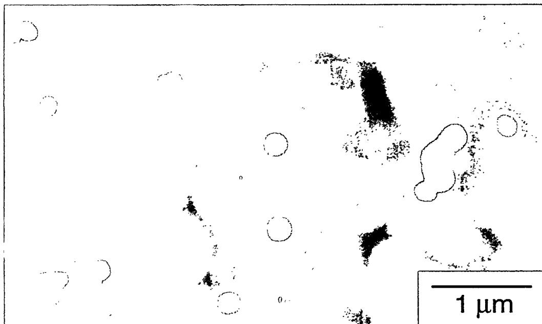
Figure 1 - Plan view SEM micrograph of coating produced with 2.5 mole %  $\text{YO}_{1.5}$  solution and total reagent concentration of 0.005 M.
