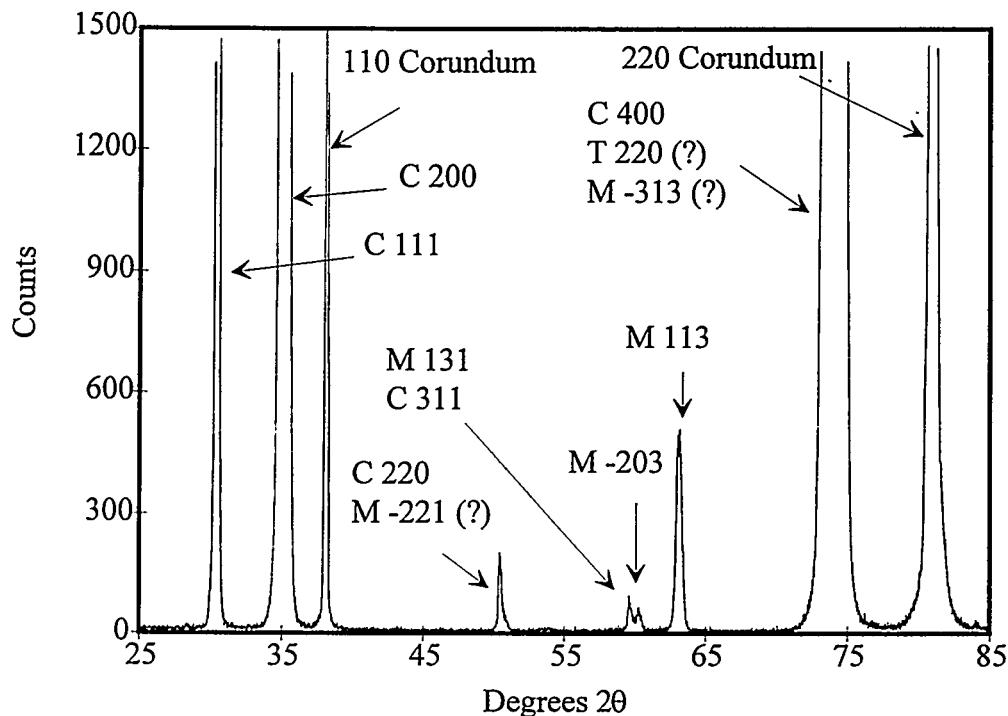
Figure 4 - X-ray diffraction pattern of coating produced with 7.5 mole %  $\text{YO}_{1.5}$  solution and total reagent concentration of 0.005 M.
