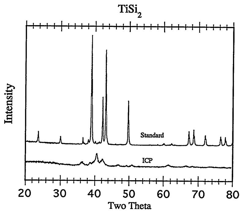
Figure 3. X-ray scan of Ti-Si compound.
