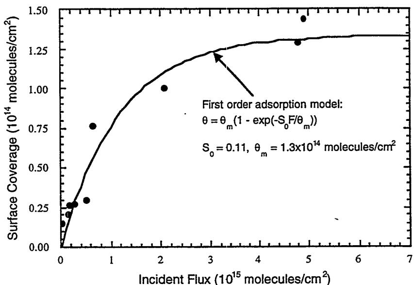
**Figure 4:** Comparison of the amount of desorbed HCl (as determined from the surface coverage) as a function of incident HCl flux. A first-order adsorption model indicates that the HCl sticking coefficient is 0.11 at 298 K.
