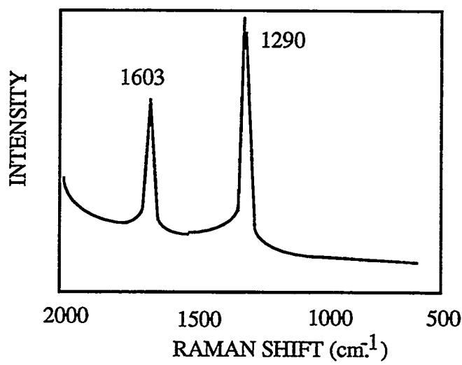
**Figure 10.** Raman spectra of matrix material produced by inverted gradient process.
