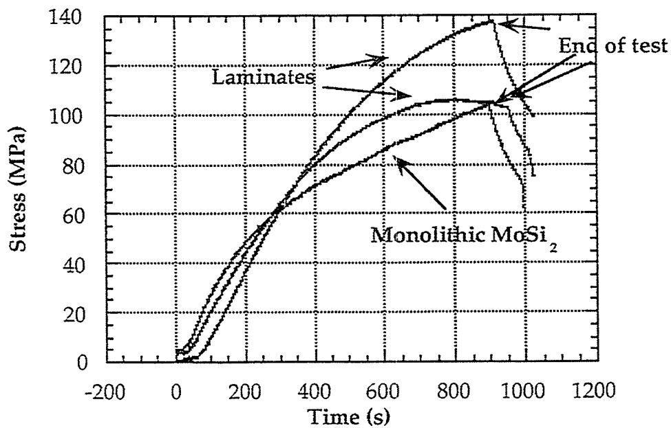
Fig. 6 Stress-time curves for MoSi<sub>2</sub>/Al<sub>2</sub>O<sub>3</sub> beams tested at 1200°C. A curve for monolithic plasma sprayed MoSi<sub>2</sub> is shown for comparison.
