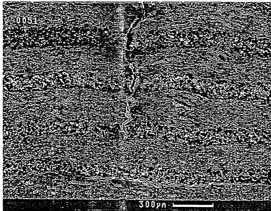
Fig. 8 Dominant crack advancing in the  $\text{MoSi}_2/\text{Al}_2\text{O}_3$  beam tested at 1200°C. Note that interface debonding does not accompany crack growth.
