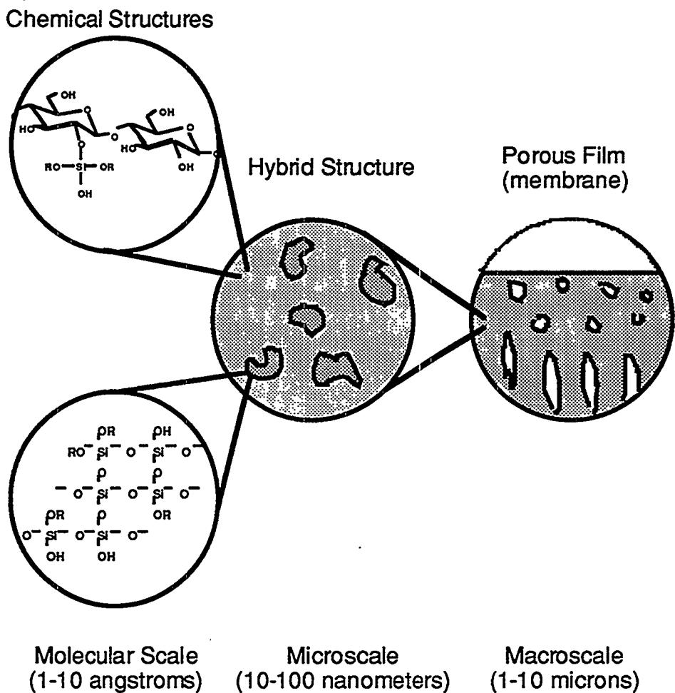
Figure 1. Schematic of the morphology of CA OIH materials.
