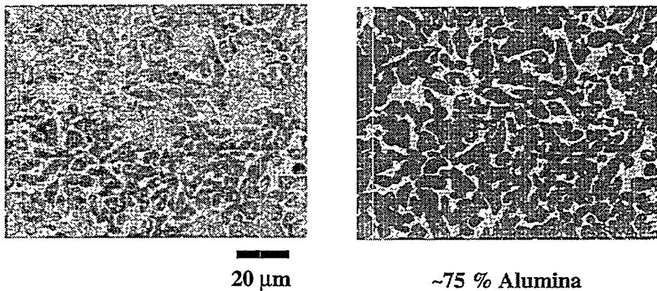
Figure 9. Optical micrograph of a ceramic-metal composite formed by aluminum penetration of and reaction with a mullite-glass preform (left). Phase concentration analysis by quantitative stereology was conducted on the digitized microstructure (right).  $\text{Al}_2\text{O}_3$  is the darker phase.
