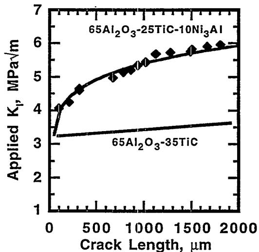
Figure 1. The fracture resistance rises rapidly with crack extension in the intermetallic-bonded composite. In comparison, neither the alumina nor the alumina-TiC composite exhibit significant fracture resistance.
