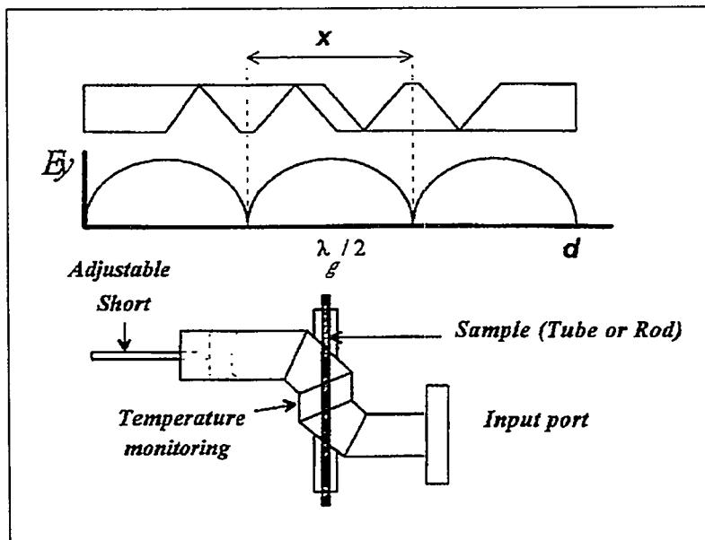
Figure 4: Schematic of Double Mitered Bend Cavity
