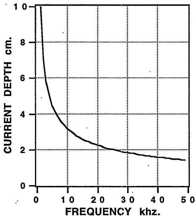
Figure 2. Variation of current depth with frequency for carbon fiber preform.
