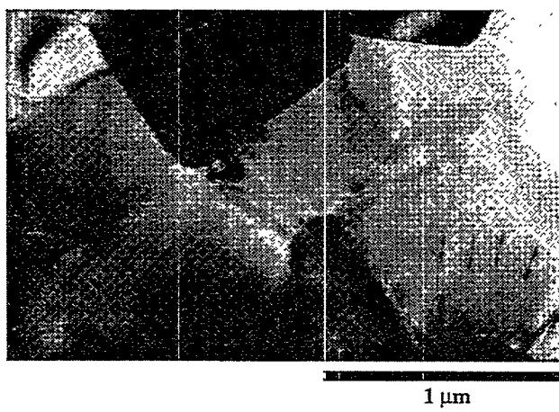
Figure 3. TEM of partially infiltrated mullite showing alumina penetration of the mullite ceramic along grain boundaries.
