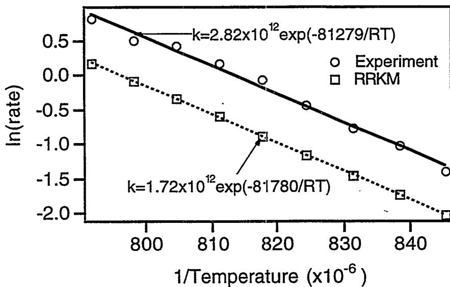
**Figure 2:** Comparison of MTS decomposition rates measured in the HTFR compared with the predictions of RRKM theory.
