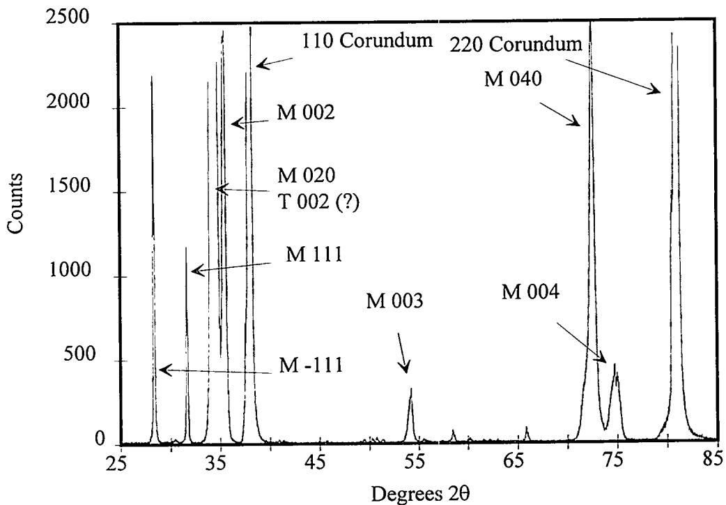
Figure 3 - X-ray diffraction pattern of coating produced with 2.5 mole %  $\text{YO}_{1.5}$  solution and total reagent concentration of 0.005 M.
