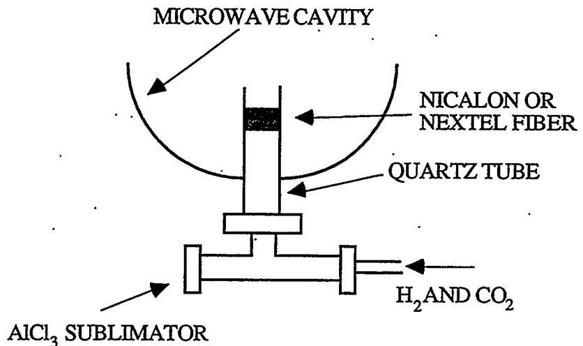
**Figure 12.** Schematic of the MACVI set-up for alumina infiltration.
