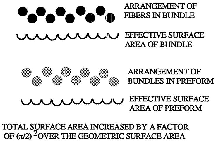
**Figure 8.** Approximate increase in surface area over the geometric surface area of a carbon fiber preform
