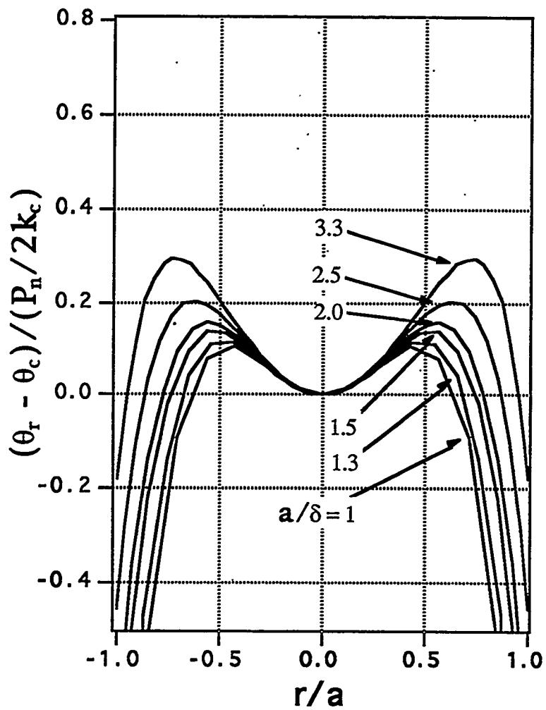
**Figure 4.** Effect of varying the relative current depth on the temperature distribution
