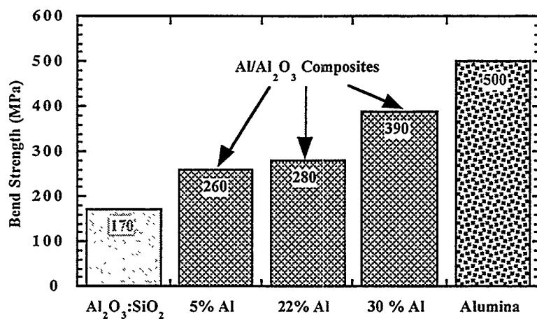
Figure 14. Bend strengths of reactively-formed ceramic-metal composites containing 5-30 volume percent aluminum compared to slip cast aluminosilicate ceramic preforms and a typical structural alumina.
