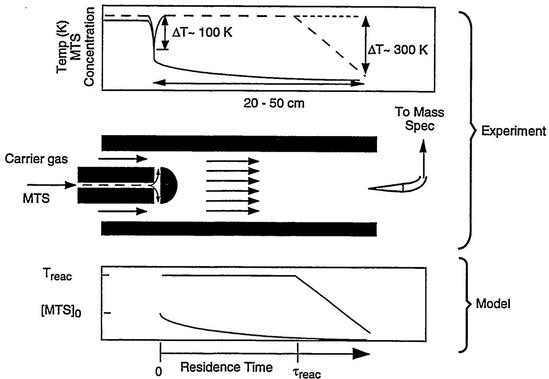
**Figure 1:** Schematic diagram of the HTFR experiment and comparison with the temperature profile used in the numerical model. Solid curves represent MTS concentration profiles, dashed curves are the temperature profiles.
