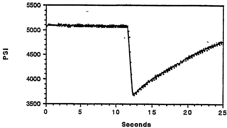
Figure 2. Data acquired during autogenous laser welding of alloy IC-221M.
