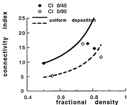
Figure 3: Connectivity index as a function of fractional density in the  $0^\circ/90^\circ$  and  $0^\circ/45^\circ$  weaves.
