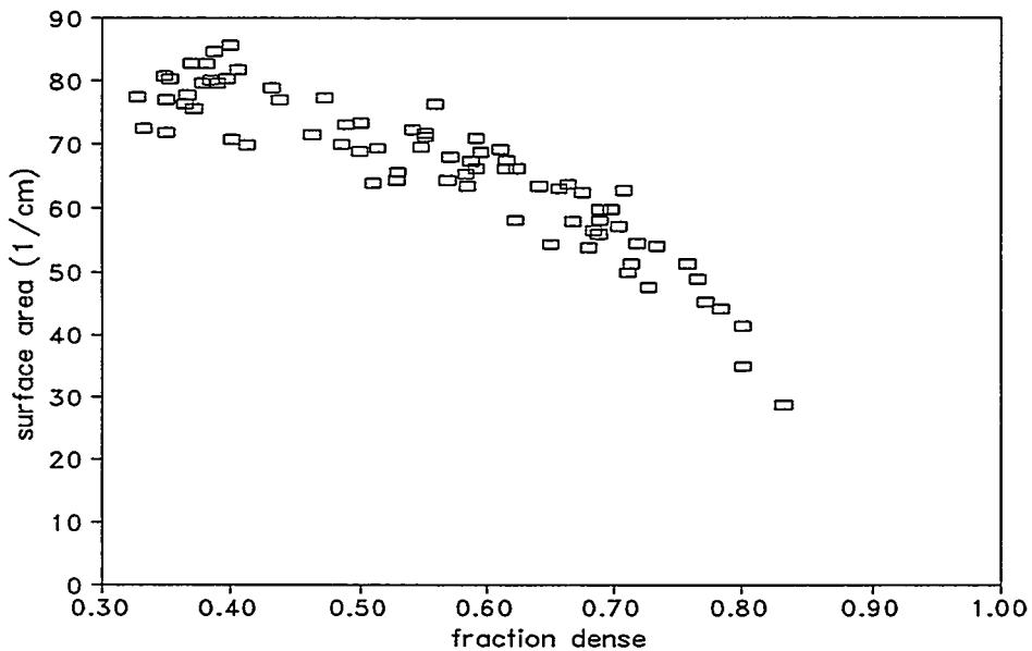
**Figure 1.** Pore surface area measured from XTM images decreases as density increases. Solid line is the estimate used previously in CVI process modeling.
