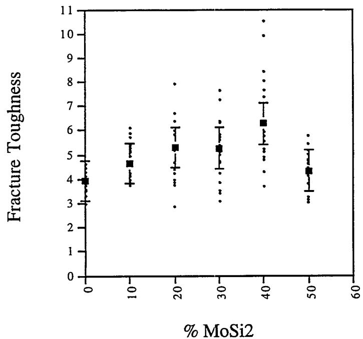
Fig. 14 Fracture toughness of  $\text{Si}_3\text{N}_4\text{MoSi}_2$  materials for 20 kg load indents.
