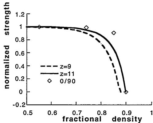
Figure 2: The normalized strength (probability of a pore belonging to the percolating cluster) for the  $0^\circ/90^\circ$  weave as a function of density. The normalized strengths of a simply connected structure (Bethe lattice) are given by the dashed and solid lines.
