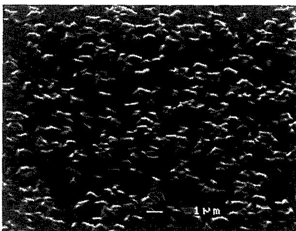
*Figure 1b:* SEM micrograph of densified film surface, tilted 50°. Note that crystal thickness (ca. 0.5 μm) is nearly that of the sol-gel film.
