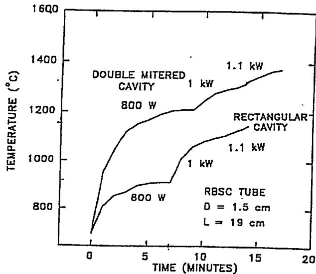
**Figure 5: Heating Profiles for Rectangular and Double Mitered Bend Cavities**
