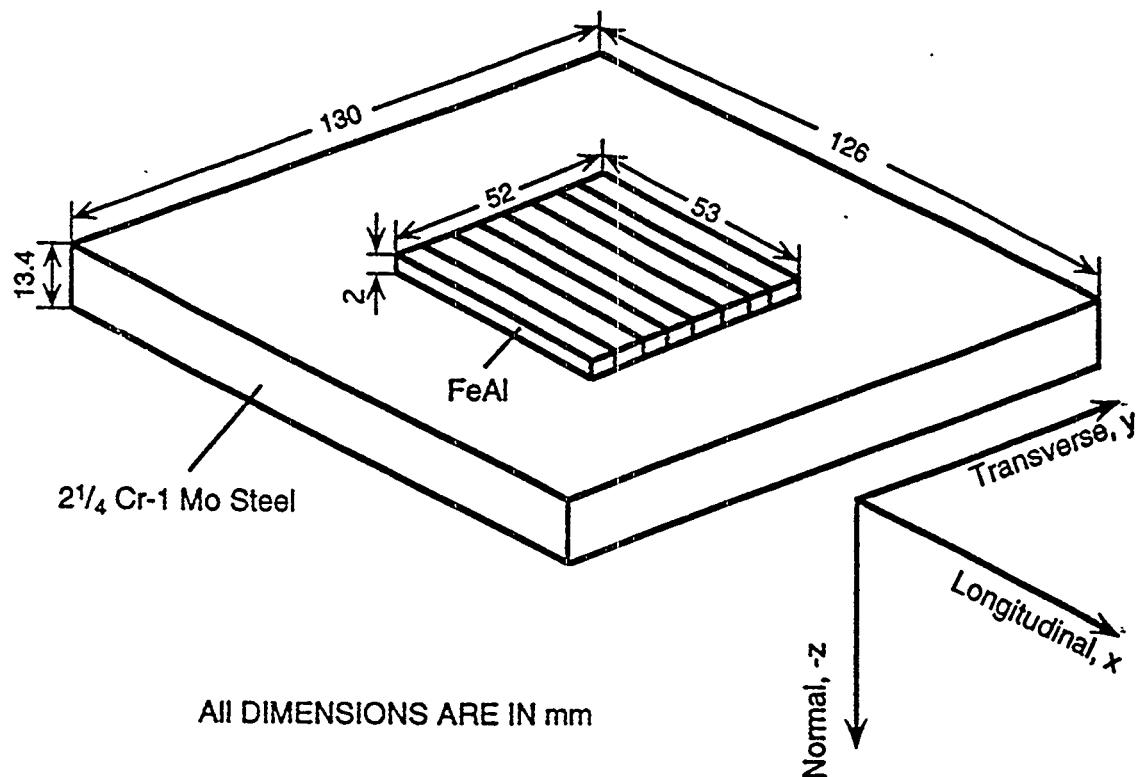
Figure 2. A schematic drawing of the FeAl weld-overlay on 2 1/4 Cr-1 Mo steel specimen used for neutron-diffraction measurements of residual stress analysis.
