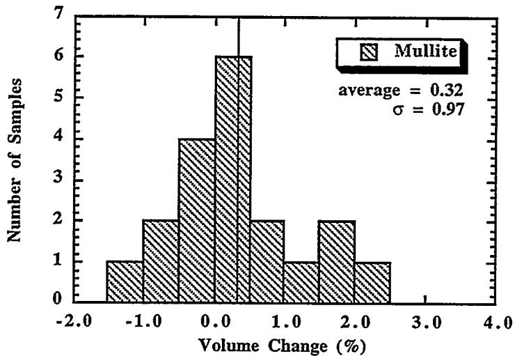
Figure 7. Measured volume changes of 17 different mullite preforms after reaction with Al to form ceramic-metal composites.
