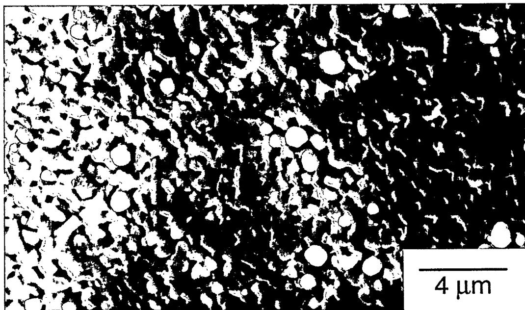
Figure 6 - Plan view SEM micrograph of coating produced with hybrid CCVD process using 5.2 mole %  $\text{YO}_{1.5}$  solution and total reagent concentration of 0.02 M.
