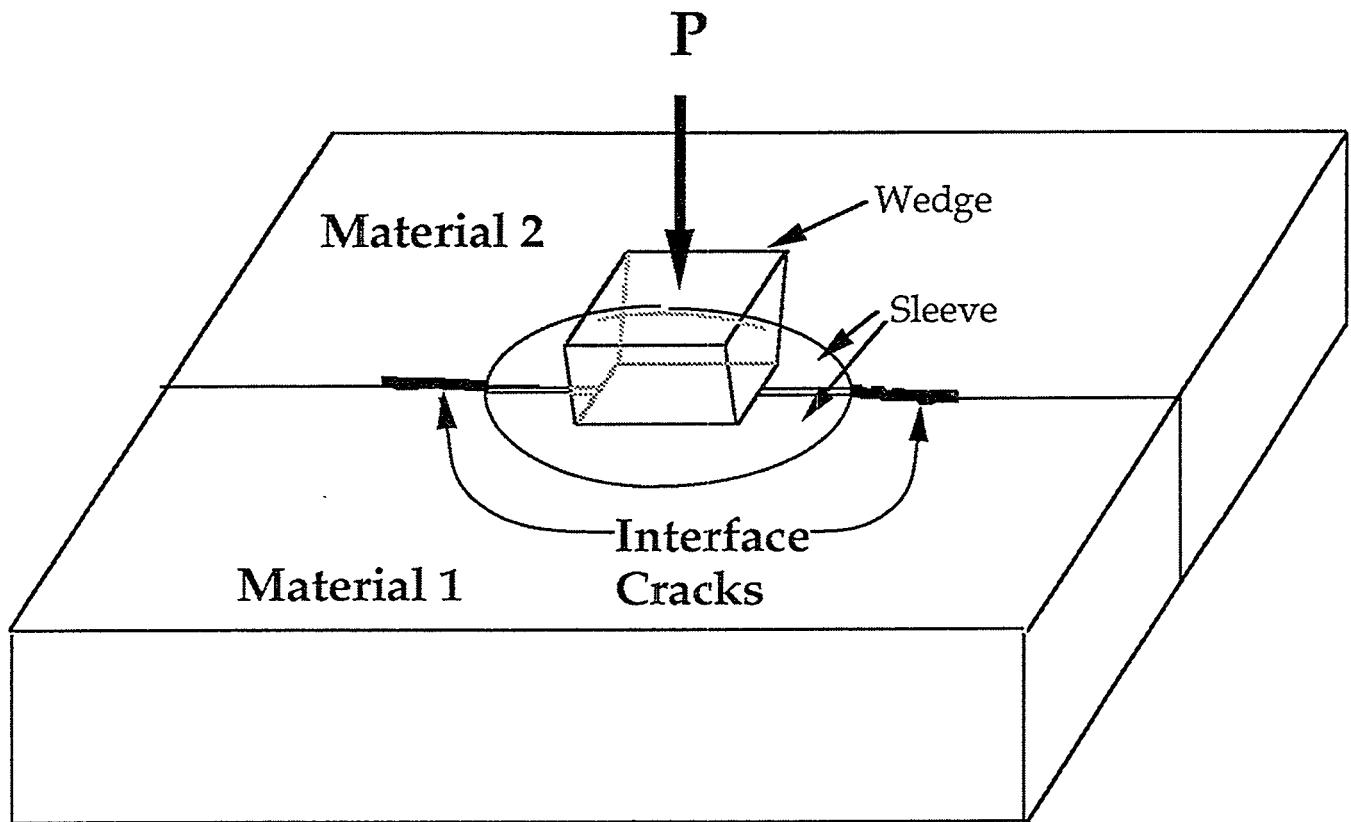
Fig. 9 Experimental set-up used in novel wedge interface toughness test.
