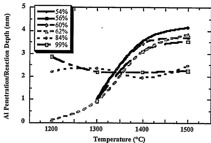
Figure 11. Al penetration and reaction depth as a function of temperature for Al reacted with mullite preforms of varying density.
