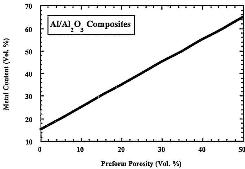
Figure 13. Predicted metal content of reactively-formed Al/Al<sub>2</sub>O<sub>3</sub> composites as a function of preform porosity.
