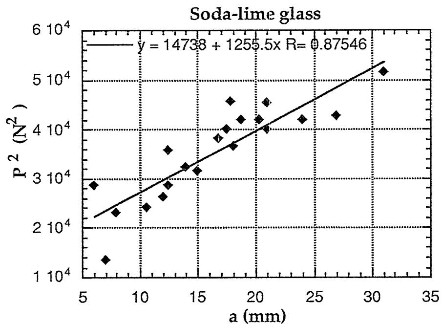
Fig. 10 Load<sup>2</sup> vs. crack length results for soda-lime glass tested by wedge method.
