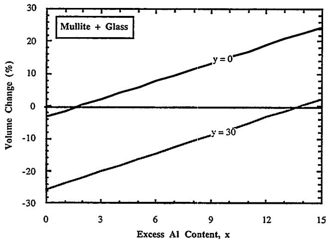
Figure 6. The calculated volume change of the mullite-glass preform when reacted with Al to form a ceramic-metal composite. Results are plotted as a function of composite Al content,  $x$ , assuming no silicon loss ( $y = 6$ ) and complete silicon loss ( $y = 0$ ) following Reaction 4.
