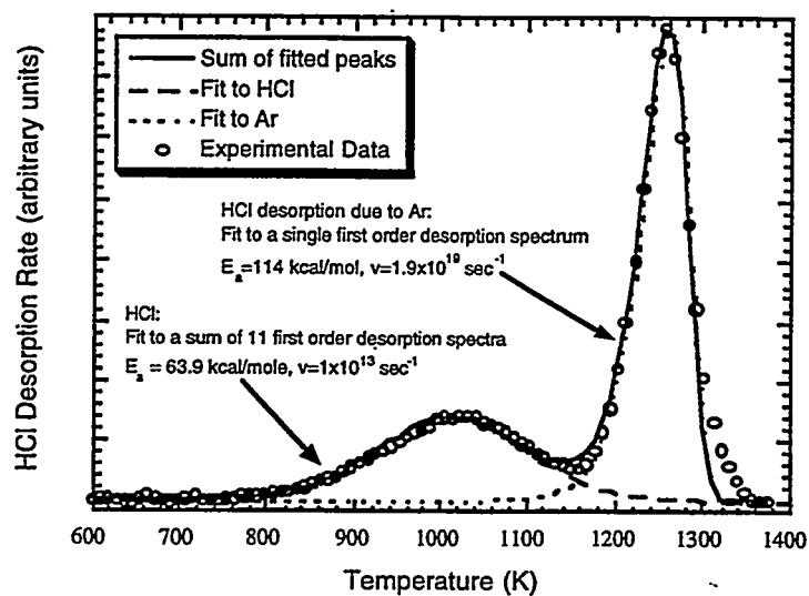
**Figure 3:** Temperature-programmed desorption profiles showing the desorption of HCl and Ar from a polycrystalline SiC surface.
