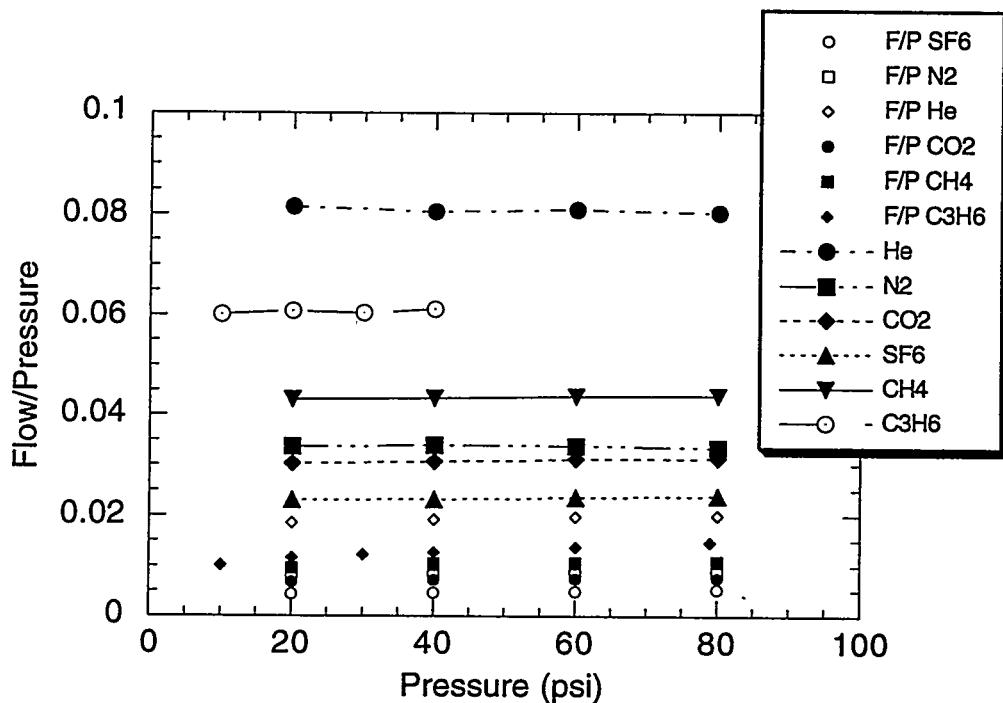
**Figure 2:** Permeation results for a  $\gamma$ -Al<sub>2</sub>O<sub>3</sub> membrane (U.S. Filter), before and after coating with a sol-gel derived zeolite film. Unconnected points are flow/pressure values for the membrane before coating, and connected points correspond to flow rates of the coated membrane. The separation factors for both the coated and uncoated membrane are Knudsen-limited.
