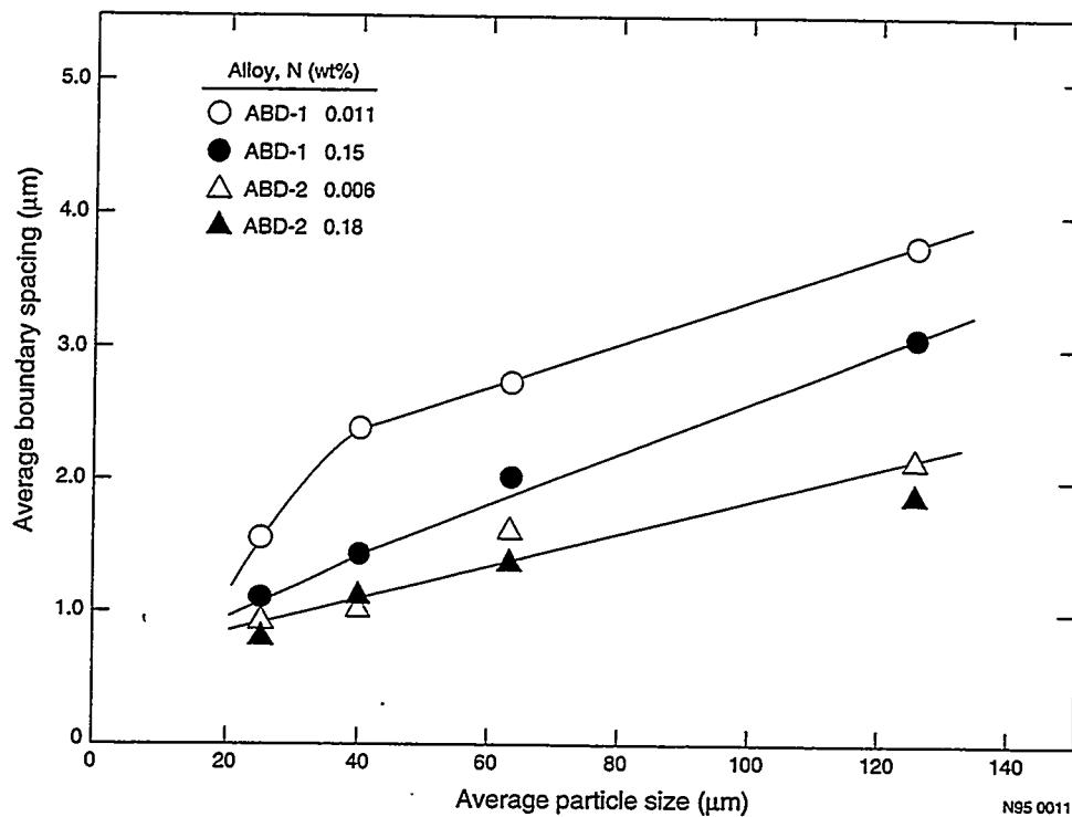
Fig. 1 – Influence of particle size on the solidification boundary spacing for ABD1 and ABD2 powders with different nitrogen contents.
