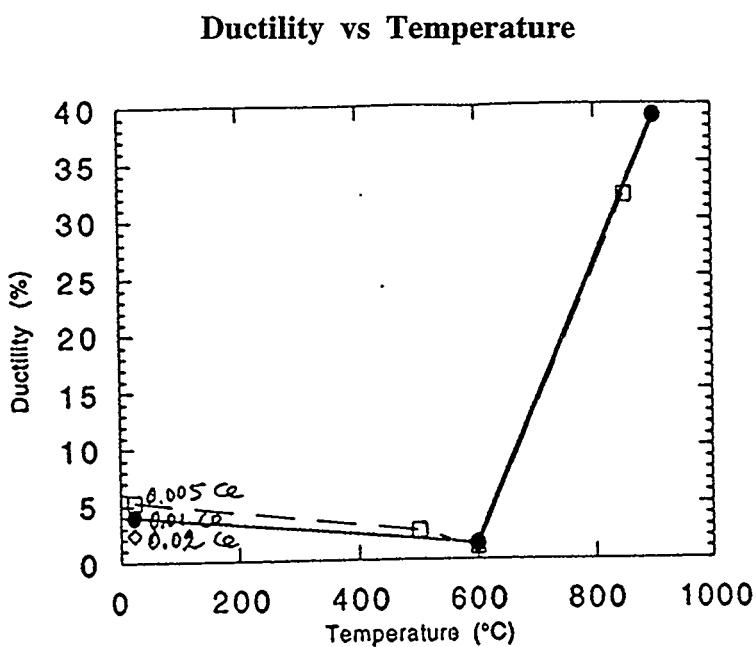
Fig. 1. The plot of tensile ductility as a function of temperature for  $\text{Ni}_3\text{Si}$  alloys doped with cerium.
