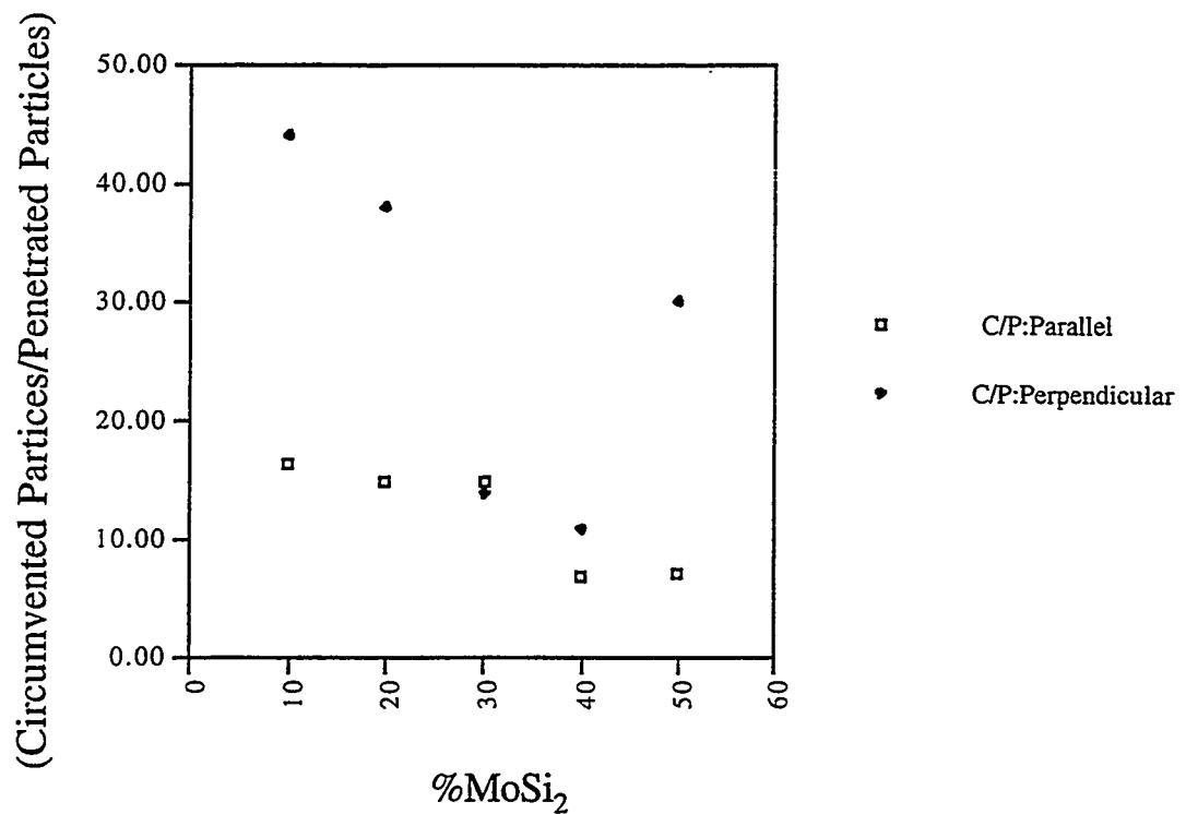
Fig. 15 Ratio of circumvented MoSi<sub>2</sub> particles and penetrated MoSi<sub>2</sub> particles for each direction.
