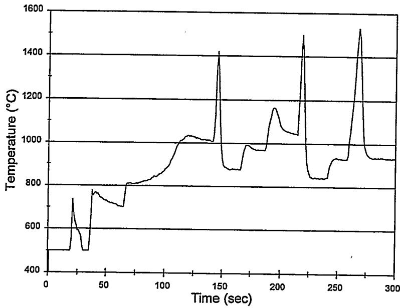
Figure 1a. Burst heating in a stationary Nextel 550 tow in a  $TE_{103}$  cavity. The microwave power was increased by step amounts, indicated by a sudden temperature rise.
