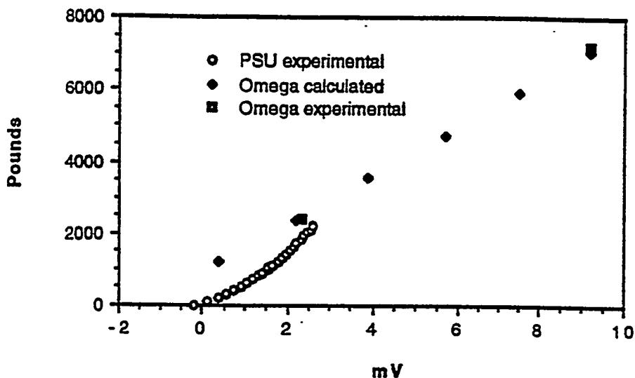
Figure 1. Calibration curve for the Omega strain bolt.
