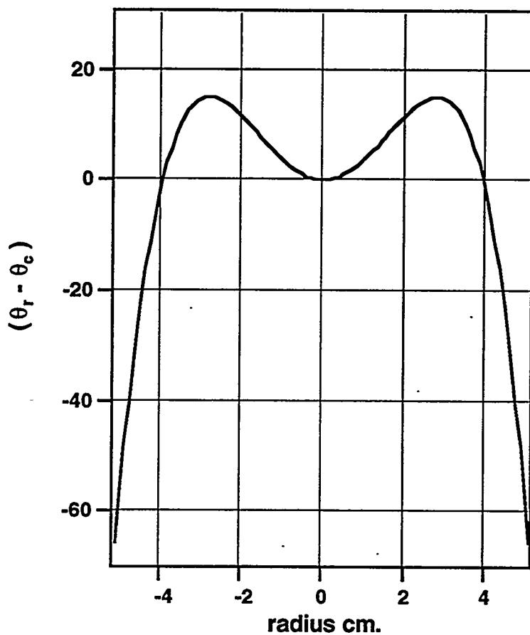
**Figure 9.** Predicted temperature gradients for a 10 cm. diameter carbon preform processed at 10 kHz.
