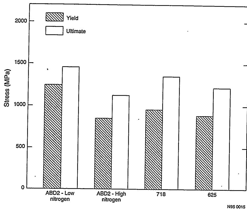
Fig. 4 – Tensile stress comparisons for age-hardenable ABD2, 718, and 625 nickel-base alloys.
