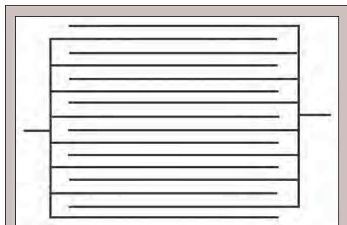
Figure 1. Schematic of the electrostatic dust detector is not drawn to scale. Particles falling in between the traces cause a temporary short circuit, which creates a voltage pulse that is recorded and related to the mass of incident dust.
