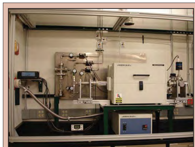
Figure 2. Photograph of the custom-built chemical vapor deposition system.
