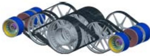
Figure 6: Summary of optimal two-stage topology based on aggressive design rules.
