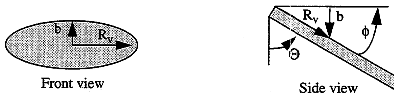
Figure 3.5-18 Two views of a partially open flapper valve.
