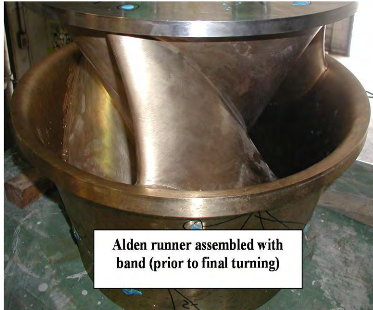
Figure 1-3 Photo of Assembled Model Turbine Runner with Band (prior to testing)
