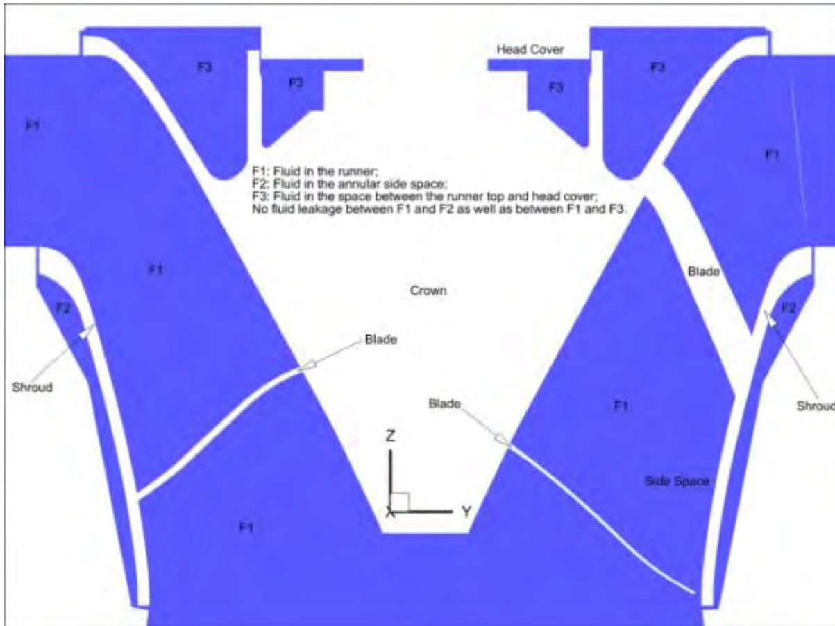
Figure 5-7 The Annular Space between the Outer Runner Shroud and the Casing, and Space between the Runner Top and the Head Cover
