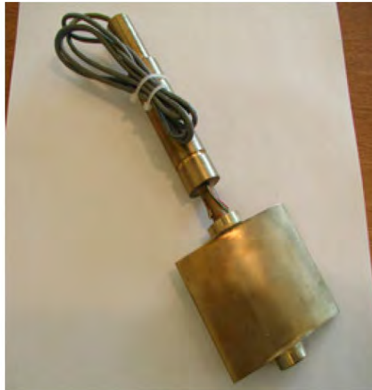
Fig. 19 – Wicket Gate Instrumented with Strain Gage for Gate Torque Measurement
