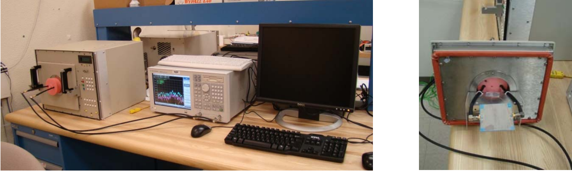
Figure 4. f_r test setup, and the mounting of a SL resonator panel.
