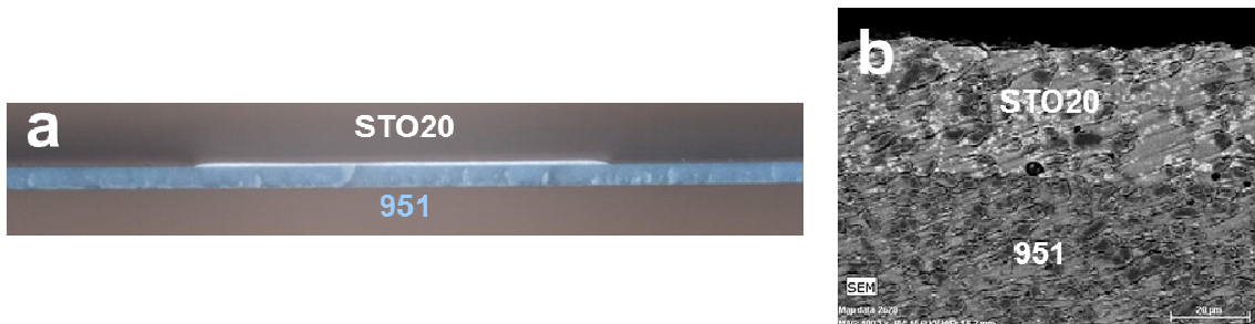
Figure 9. a) Optical cross section of sintered CMB STO20 on 951, and b) a SEM cross section of the interface between the CMB STO20 and the 951 LTCC.
