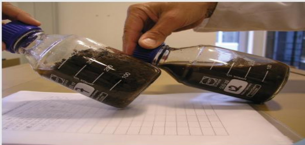
Washed pWS before (left) and after (right) hydrolysis.
