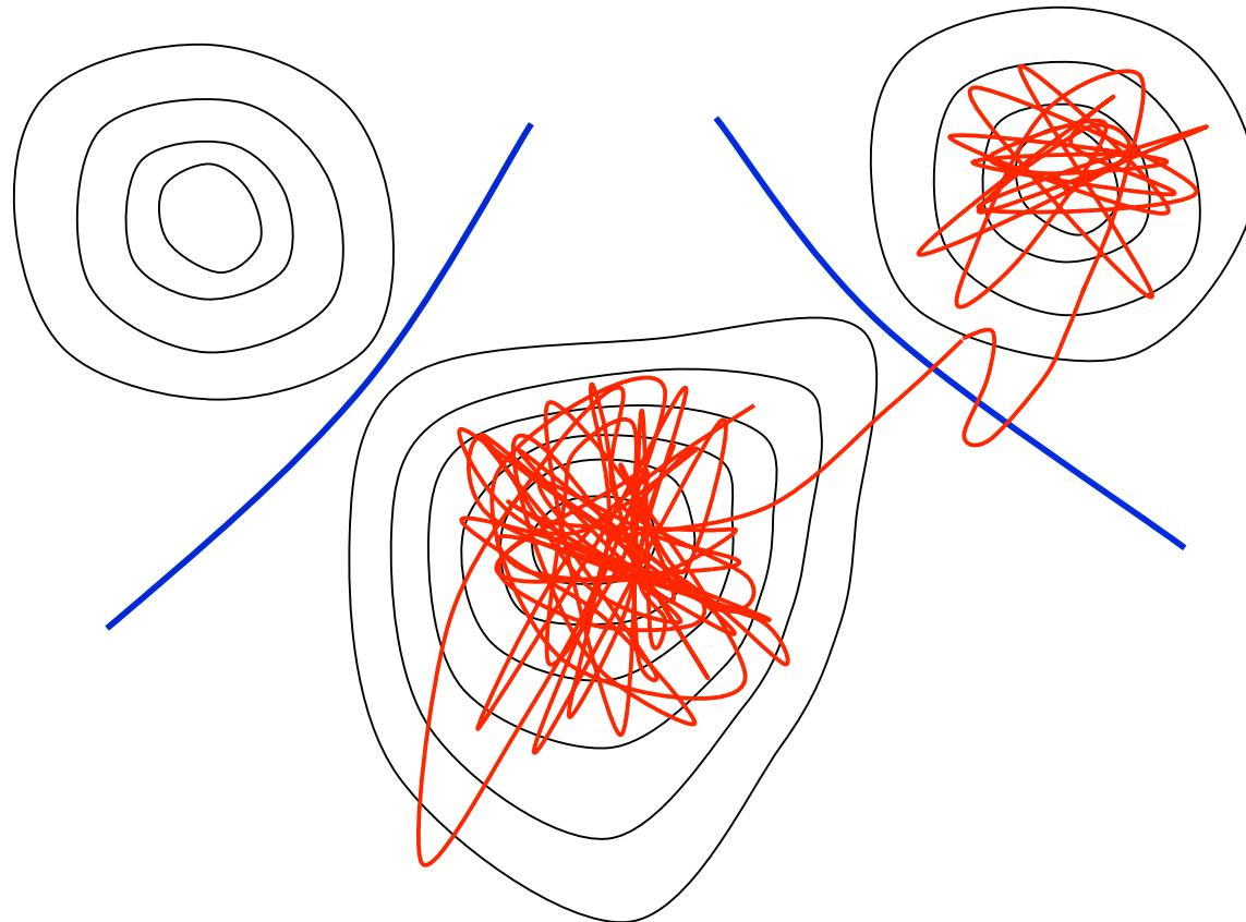
An infrequent-event system vibrates in  $3N$ -dimensional basin many times before finding an escape path. The trajectory finds an appropriate way out (i.e., proportional to the rate constant) without knowing about any of the escape paths except the one it first sees. *In the AMD methods, we exploit this property, letting the trajectory find an appropriate escape path, but we carefully trick it into doing this more quickly.*
