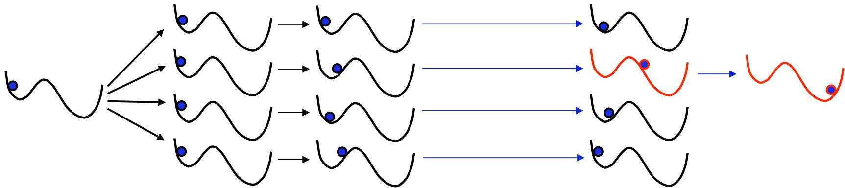
The summed time ( $t_{\text{sum}}$ ) obeys the correct exponential distribution, and the system escapes to an appropriate state.
