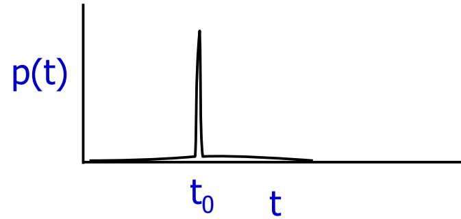
If  $p(t)=\delta(t-t_0)$ , parallel replica simulation will detect an event on all  $M$  processors at the same time ( $t_0$ ), giving no boost. Worse, the summed time will predict a transition time too large by exactly a factor of  $M$ .
