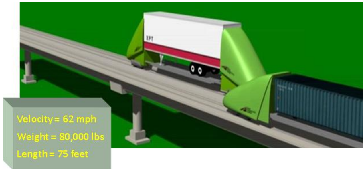
Freight Shuttle transporters operating on elevated, bi-directional guideway.
