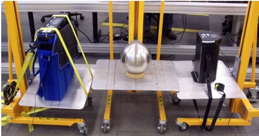
Experiment Setup for one and one half inch steel moderator, one half meter off the ground and one half meter from source
