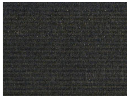
Figure 28 Crystalline Particles Found on Anode GDL on Cell Disassembly
