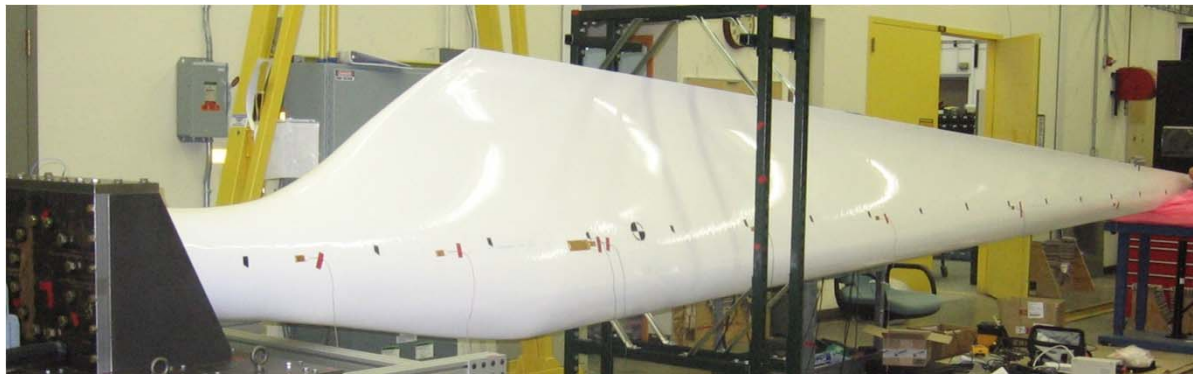
Sandia's 9-meter CX-100 Composite Blade
