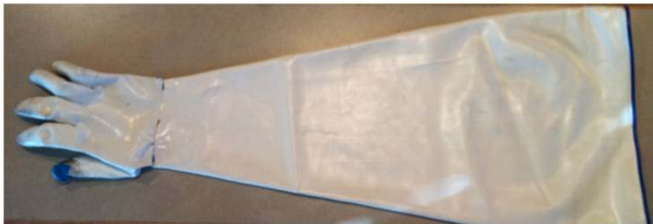
Figure 9 Picture of the prototype glove glued to a glove sleeve to make a whole glovebox glove.
