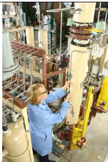
Figure 14 Absorber Column Prior to Heat Tracing and Insulation of Tubing/Piping
