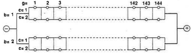
Figure 6. Equivalent Circuit of GPHS RTG
