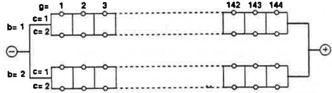
Figure 6. Equivalent Circuit of GPHS RTG
