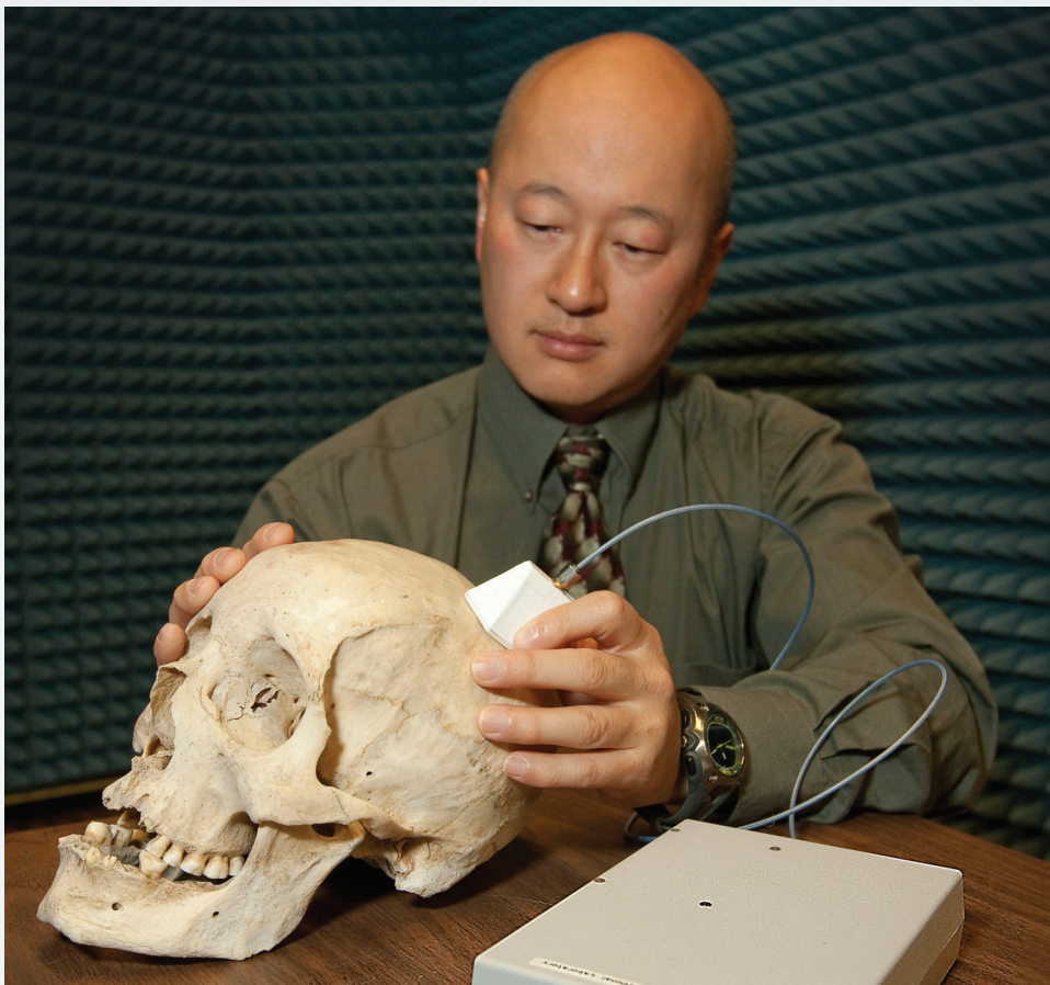
LDRD researcher John Chang tests a prototype intracranial hematoma detector on a human skull. Work on this project won an award for excellence in technology transfer from the Federal Laboratory Consortium.
