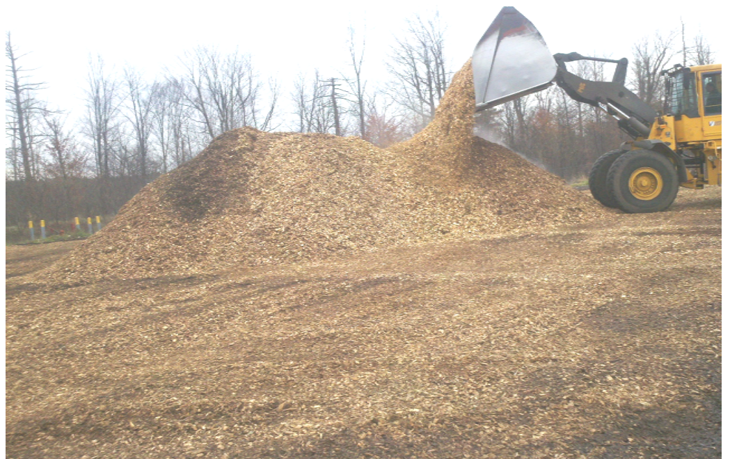
Photo 4 Fuel mixture preparation, willow and whole tree chips being turned with a front-end loader (Lyonsdale Biomass 15Nov11)
