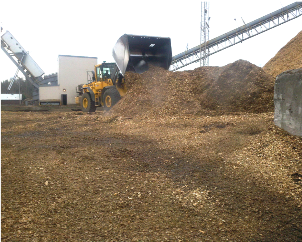
Photo 5 Blended fuel mix being arranged on Laidig reclaiming, truck dumper and stackout conveyors in background (Lyonsdale Biomass 15Nov11)
