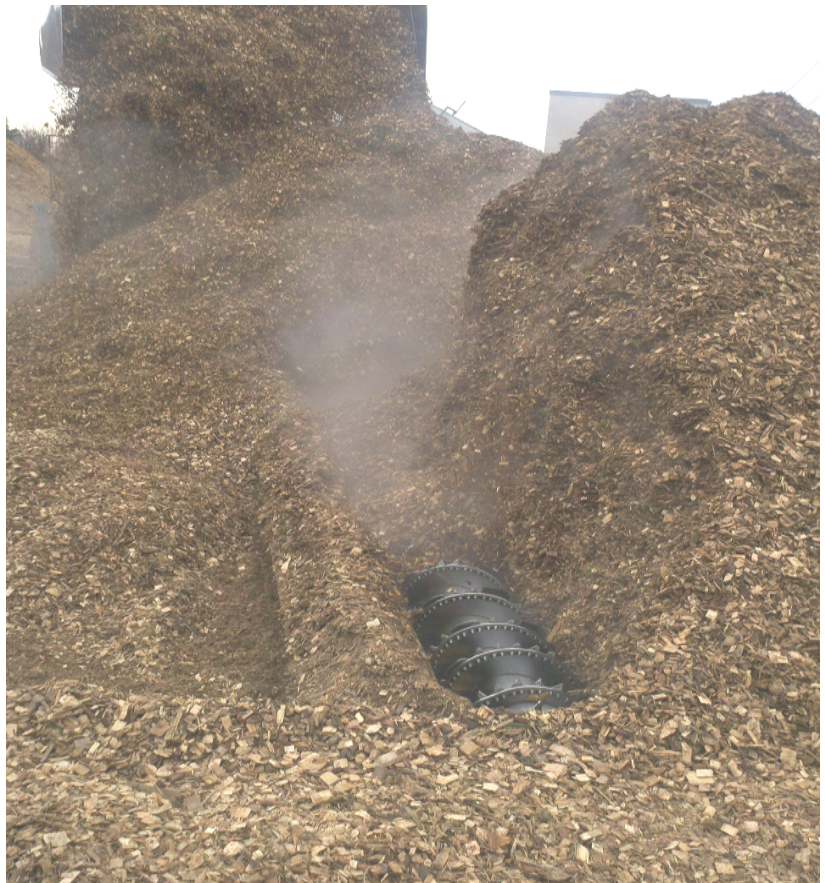
Photo 6 Fuel being reclaimed by an under-pile screw, front-end loader dumping onto pile in background (Lyonsdale Biomass 15Nov11)
