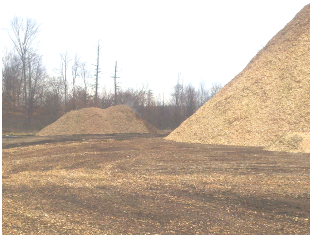
Photo 1 Lyonsdale Biomass woodyard showing willow chip pile in background, whole tree chip pile to right in foreground (15Nov11)
