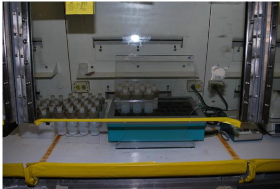
Pu oxide closed vessel acid digestion – nuclear fuel
