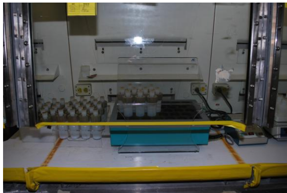
Pu oxide closed vessel acid digestion
