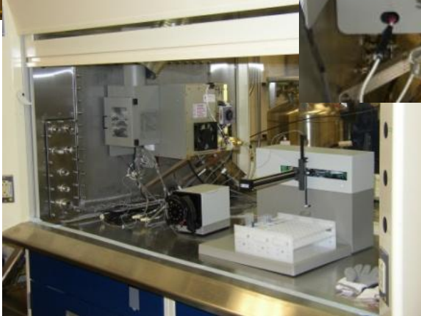
ICP-AES (Prodigy, Teledyne Leeman) interfaced with glove box
