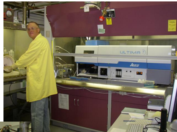
Fume hood contained ICP-AES (Ultima 2, Horiba Jobin yvon)
