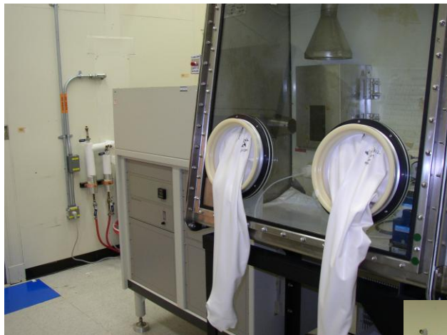
Glove box interfaced ICP-AES (IRIS, Thermo Electron)
