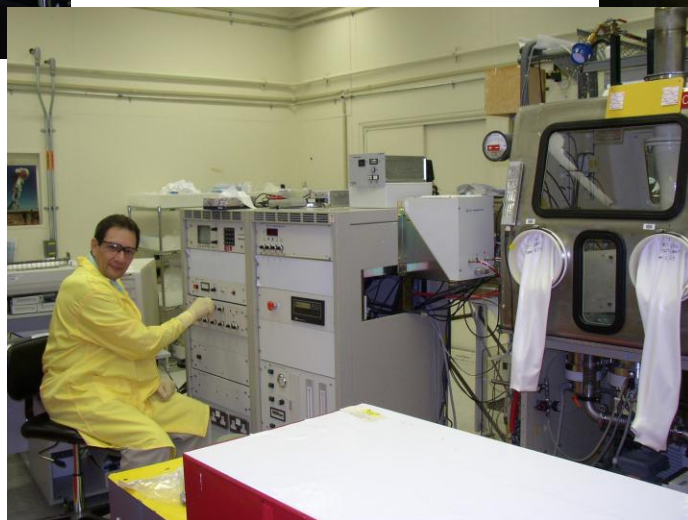
Glove box interfaced ICP-MS (VG PQ2+)
