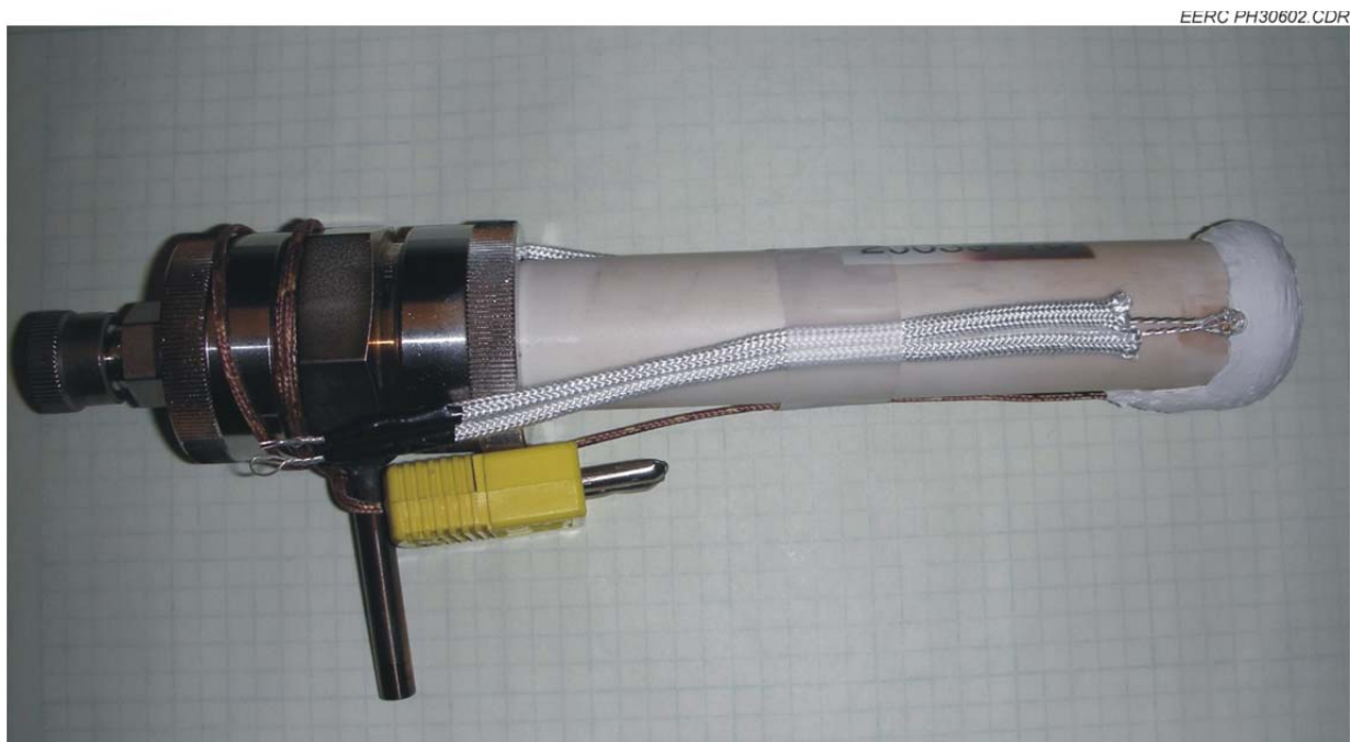
Figure 6. Test button of a Franklin Fuel Cells copper-based SOFC.
