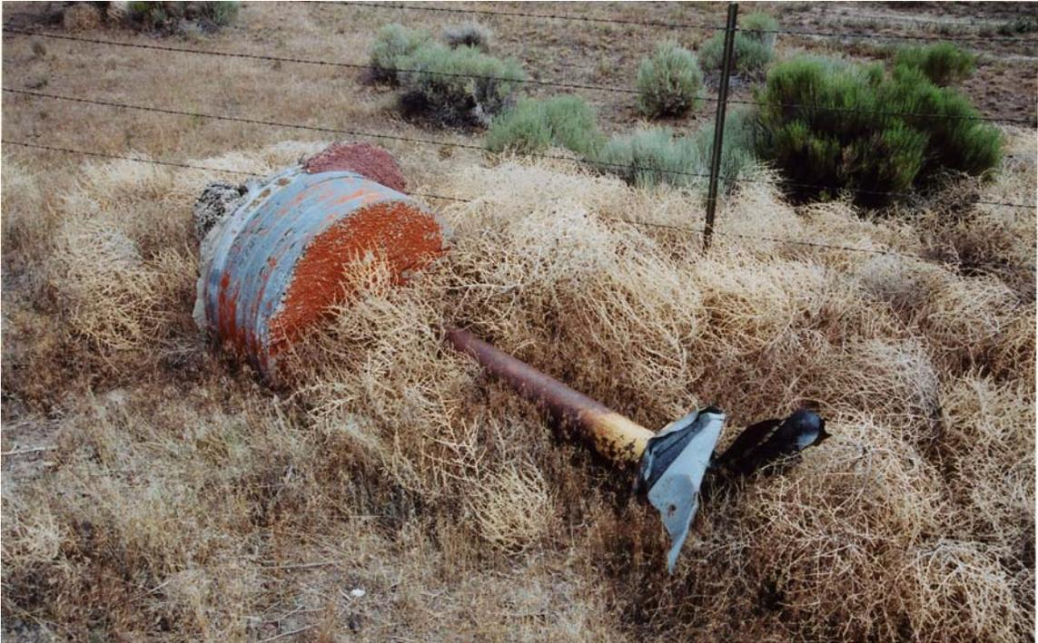
Figure 3.16-13. The surface motion targets are made of 8-inch diameter pipe with concrete-filled culvert collars. The targets were placed radially at varying distances from ground zero and recorded with motion picture cameras (photo taken July 2004 on file at Desert Research Institute).
