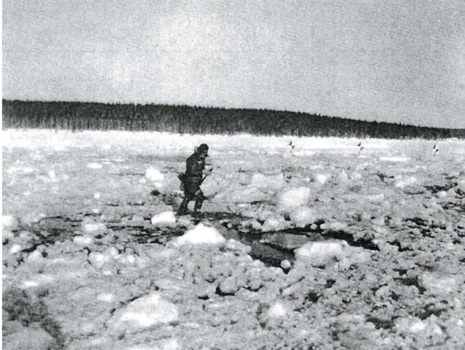
Figure 3.10-3. View of Operation Breakup yield scaling shot, Shot 31- a 940 pound charge was used (Kurtz 1966, Figure 4.11).
