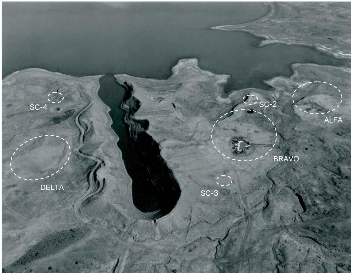
Figure 3.15-14. The Pre-Gondola project site after remediation work conducted in the summer of 1972. The Alfa, Bravo, and Delta craters have been backfilled while the small calibration craters SC-2, SC-3, and SC-4 were not filled. Photo taken Sept. 27, 1973 (adapted from Photo No. 904, Box 977 on file at the U.S. Army Corps of Engineers, Fort Peck Area Office, Montana).
