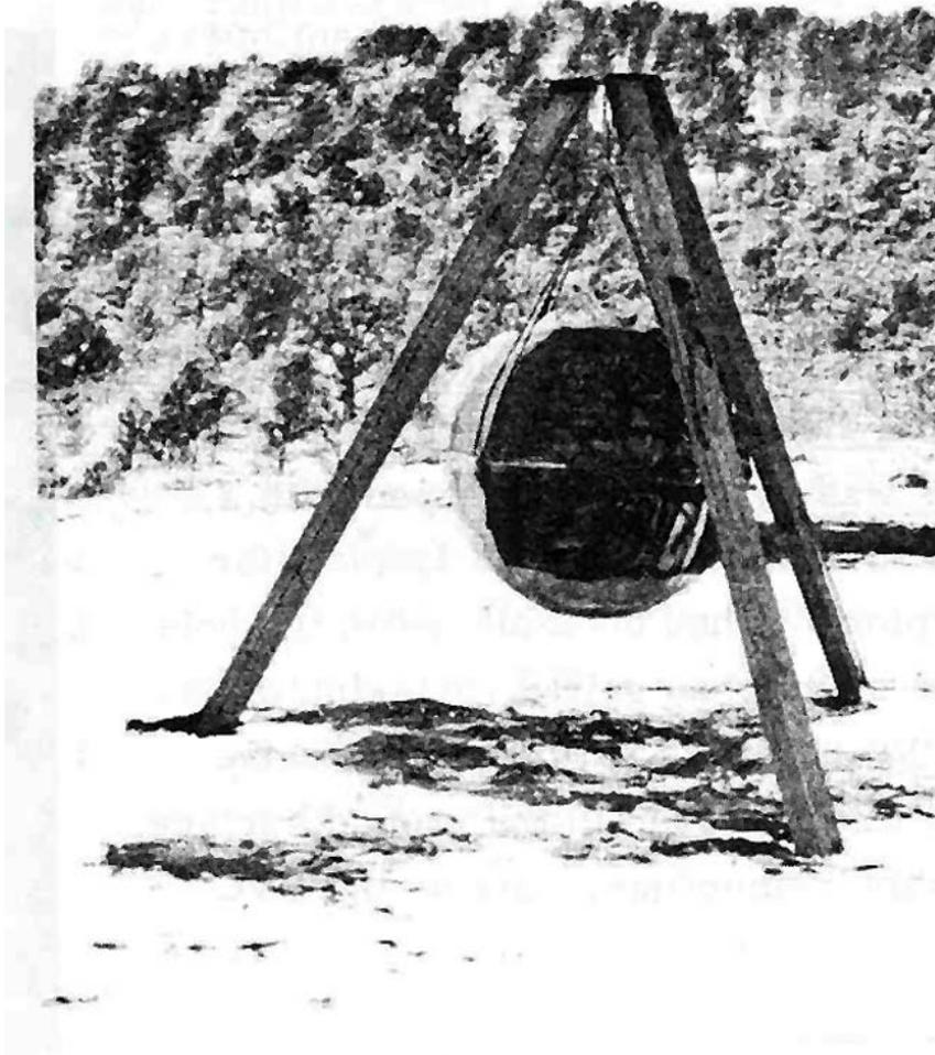
Figure 3.23-5. Suspended charge for Charge B10, Middle Course I (Fitchett 1971, Figure 7).
