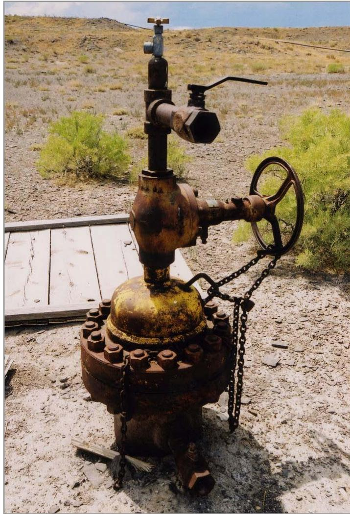
Figure 3.25-10. Close-up of the Project Utah EX-1 well head (photo taken August 2005 on file at Desert Research Institute).
