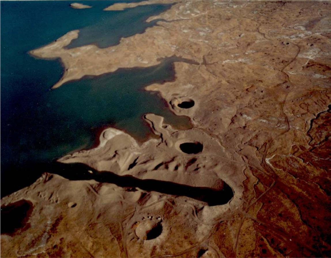
Figure 3.15-10. Aerial view of the Pre-Gondola experiment trench, Nov. 3, 1969 . The large Pre-Gondola I Alfa, Bravo, and Delta craters are clearly visible. Two of the seismic calibration craters, SC-1 and SC-4 can also be seen (Photo No. CFP70-1272 on file at the U.S. Army Corps of Engineers, Fort Peck Area Office, Montana).
