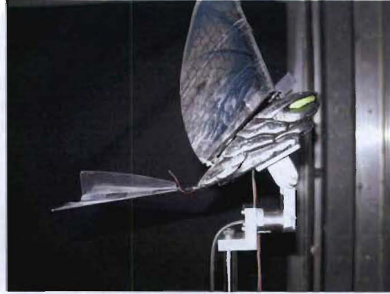
Figure 6. Force sensor mounting brackets. This image illustrates how the base plate can be rotated to obtain various angles of attack.
