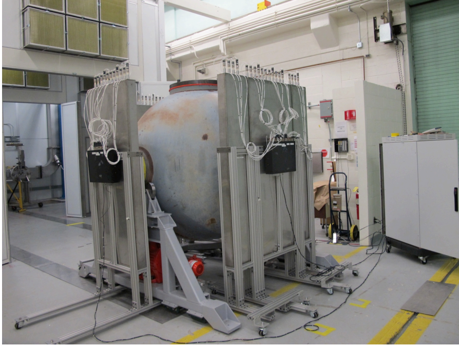
Figure 2: The CVAS positioned around an empty vessel. The polyethylene moderator has been encased in aluminum to reduce fire loading. The ends of the ^3\text{He} tubes and their preamplifiers can be seen projecting from the tops of the detector banks.
