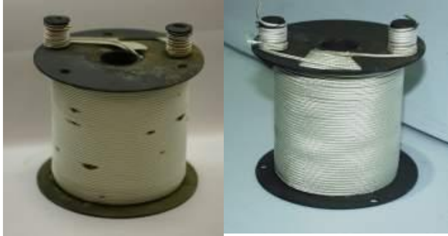
Fig 16: Barrel coil samples illustrating the elimination of leakage during processing
