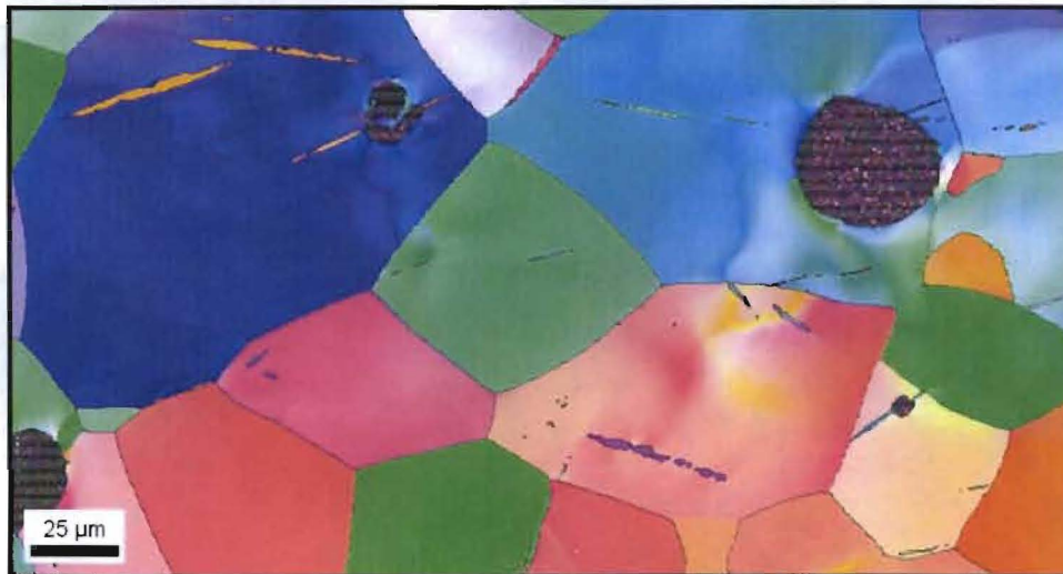
Void damage nucleated at twin boundaries
