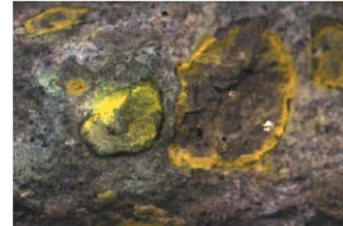
Figure 2. Image of concrete core treated with sodium cobaltinitrite and rhodamine B base solutions. Fractured core from a pavement in Albuquerque (NM) showing significant distress in the field. Treated core shows staining by sodium cobaltinitrite around reactive aggregates and within some air voids, but only minor staining by rhodamine B base. Petrographic examination using optical and electron microscopies confirmed that yellow stained material was a K-rich alkali silica gel. Image is scaled to approximately double actual size.
