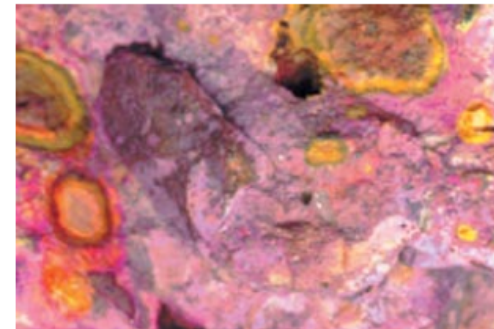
Figure 3. Image of concrete core treated with sodium cobaltinitrite and rhodamine B base solutions. Fractured core from a highway pavement in New Mexico showing severe distress in the field. Treated core shows extensive staining by both sodium cobaltinitrite and rhodamine B base. Petrographic examination using optical and electron microscopies confirmed that yellow stained material was a K-rich alkali silica gel whereas the pink-stained material included a Ca-rich, alkali-bearing silica gel. Image is scaled to approximately double actual size.
