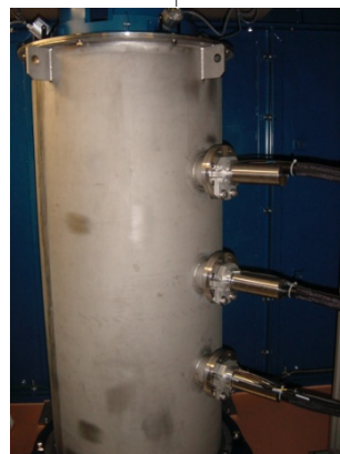
Camera Radiation Detector and Pu canister assay system installed in Japanese reprocessing facility
