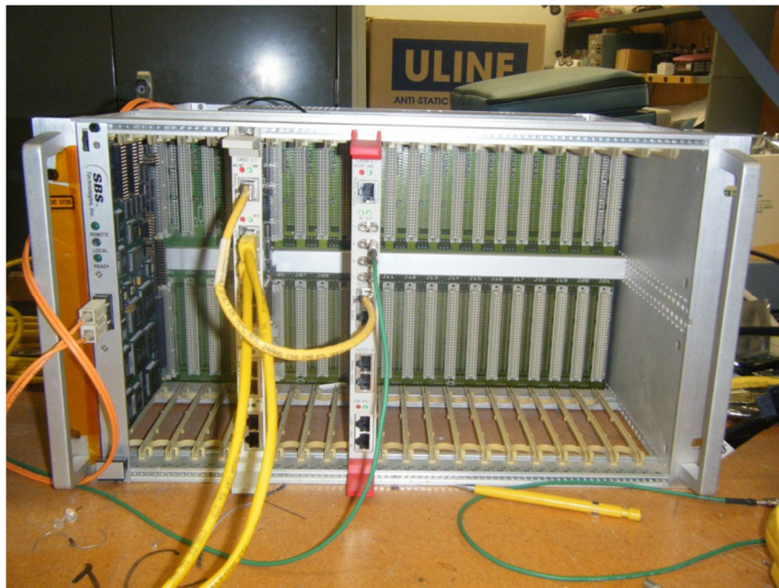
Figure 2.6: Front-end electronics: CRIM (right) and CROC (left).
