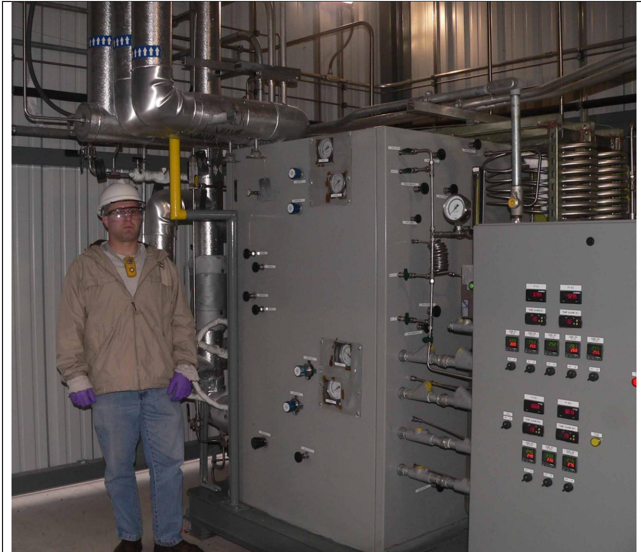
Figure 16. Full scale CMS bundle testing unit as installed at the PSDF facility. The unit is configured to accept one full scale 85-tube bundle.
