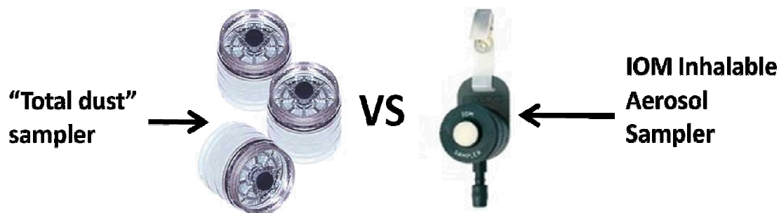
Figure 6. “Total dust” 37-mm CFC and IOM (Inhalable) samplers
