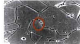
Inclusions at grain boundary
