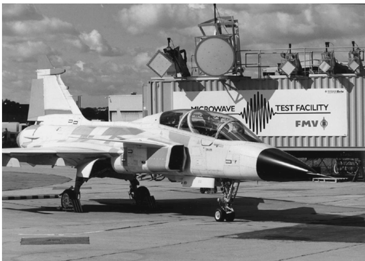
A European fighter jet undergoing HPM testing at the Swedish Microwave Test Facility.
