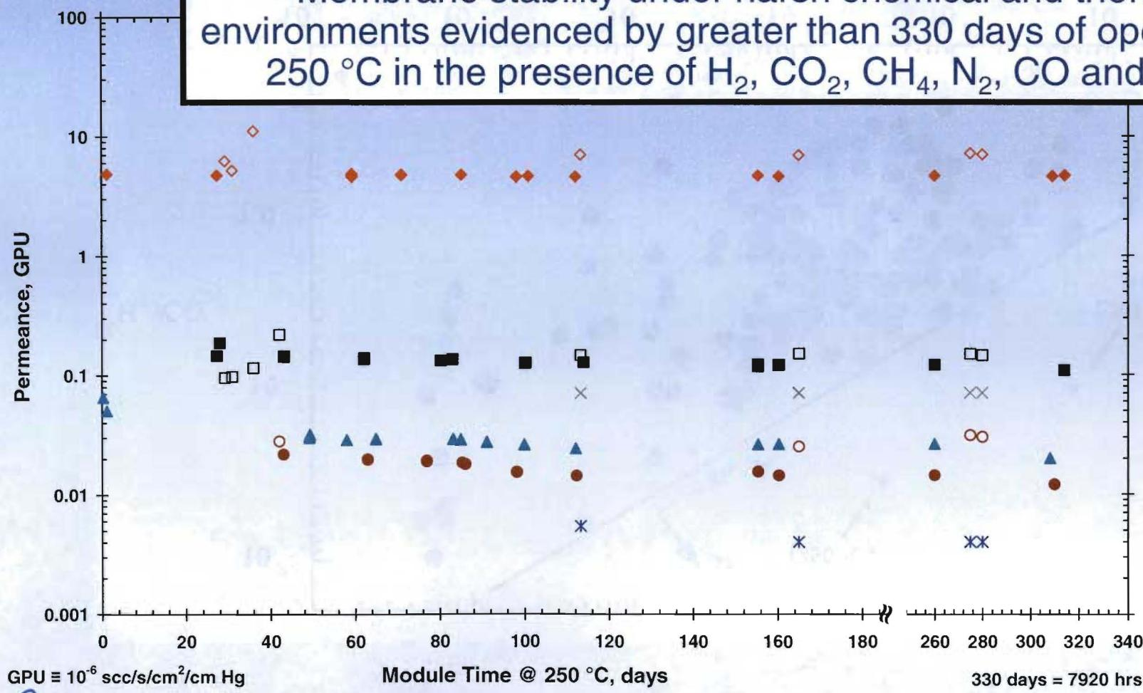
$\text{H}_2\text{S}$  is at detection limit of our analytical equipment.
