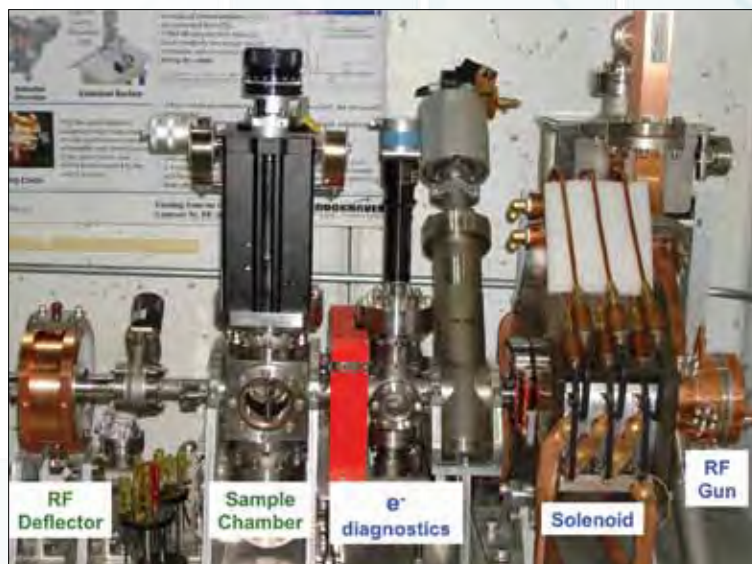
The MeV UED system installed at the NSLS SDL
