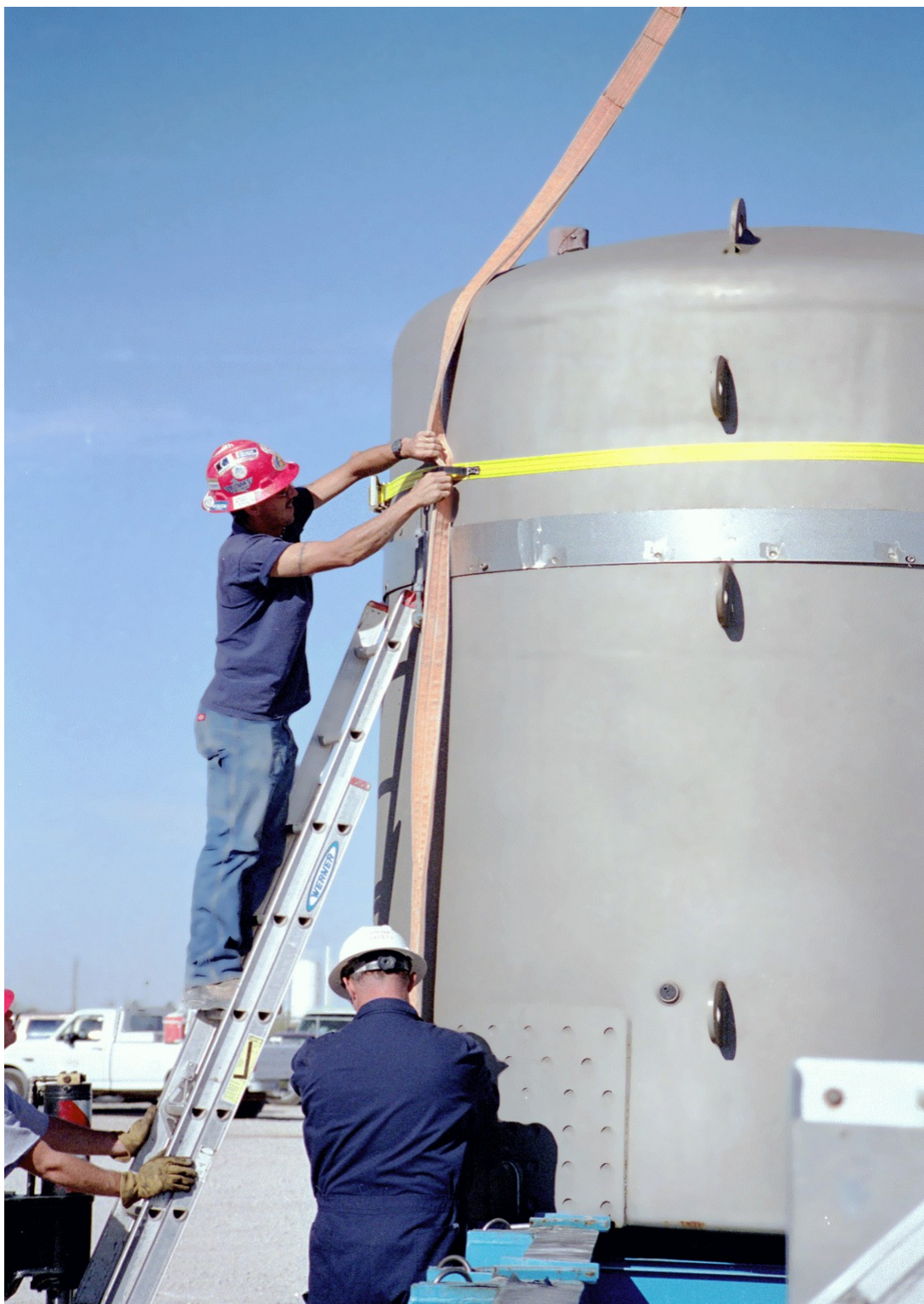
Figure 2.3-2 – Vertical Lift of a TRUPACT-II Using a Lift Sling Alignment Strap Sling is fed through the forklift pockets and up through the loops on the alignment strap.
