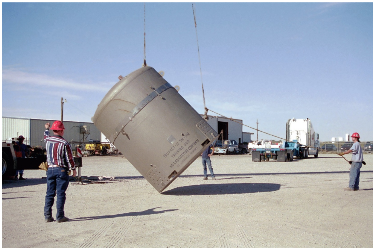
Figure 2.3-15 – TRUPACT-II Package Rotation Using Weld-On Lugs
