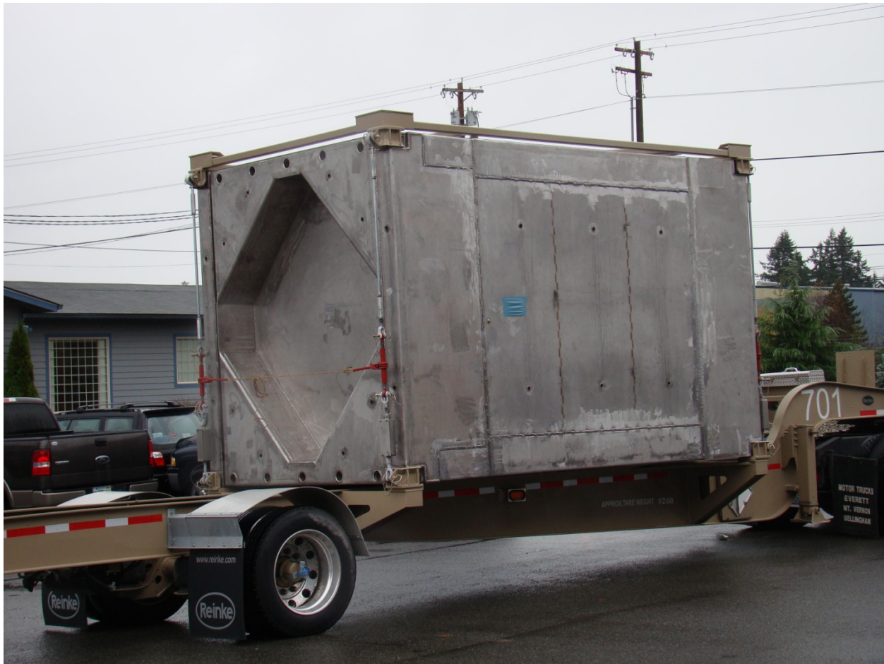
Figure 5.3.1-3 – TRUPACT-III Secured on TRUPACT-III Trailer
