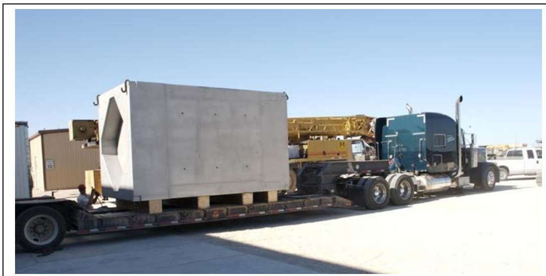
Figure 5.3.2-1 TRUPACT-III on a Lowboy Trailer Prior to Being Secured (Note ISO container lugs installed on bottom corners.)
