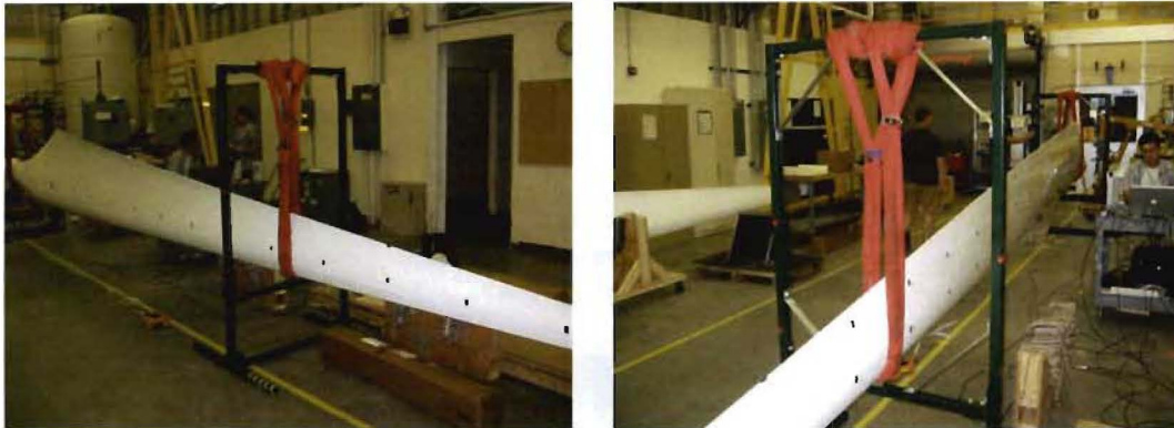
Figure 12: Frame in baseline configuration (left) versus the stiffened frame (right)
