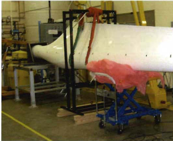
Figure 8: Free-Free II configuration with cart and packing foam supporting blade
