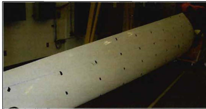
Figure 1: Measurement location grid on CX-100
