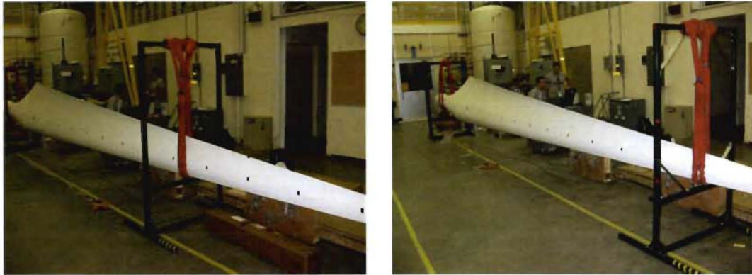
Figure 14: Tip-end frame in baseline location 6.5m from root (left) versus moving the frame to 8m from root (right)
