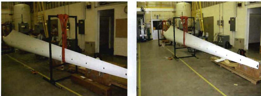
Figure 16: Tip-end frame in baseline location 6.5m from root (left) versus moving the frame to 5m from root (right)
