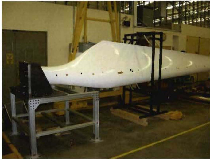
Figure 5: Blade mounted to fixture for Fixed-Free Test
