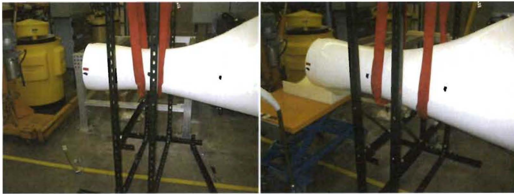
Figure 22: Root support in baseline location (left) versus moved to 0.86m from root (right)
