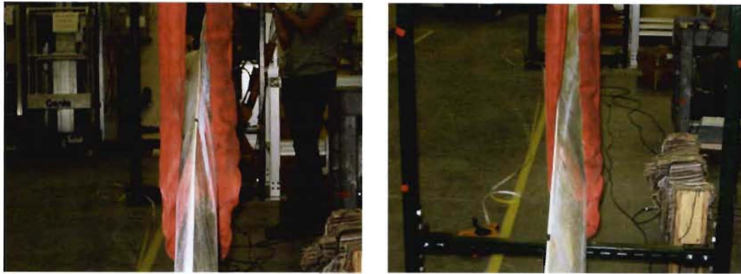
Figure 10: Blade in baseline orientation (left) versus rotated 12° orientation (right)
