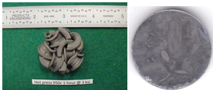
Figure 21. Cambridge titanium after consolidation by vacuum hot pressing.
