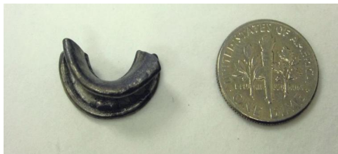
Figure 19. Cambridge process titanium.
