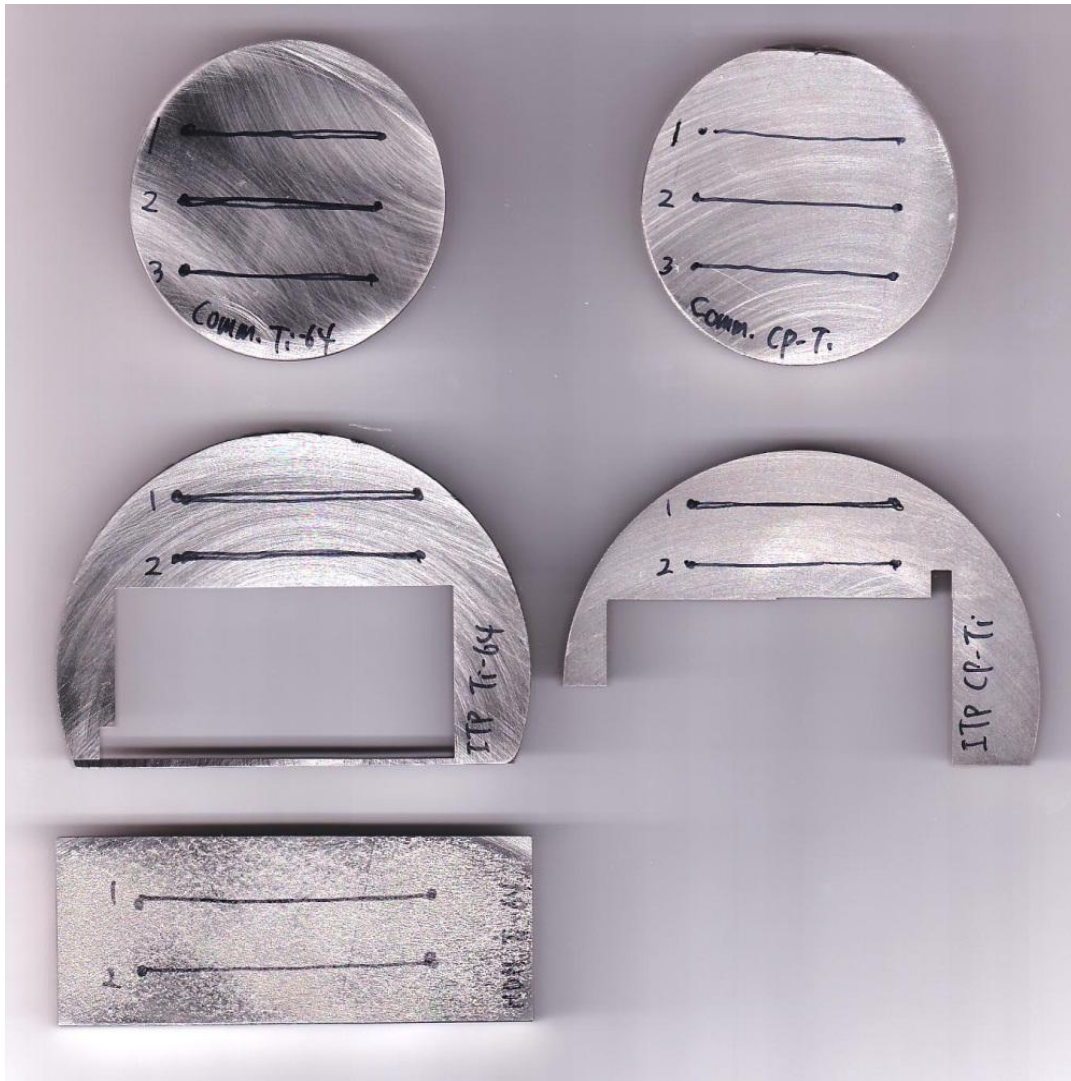
Figure 32. Electron Beam (EB) Weld Titanium Test Specimens
