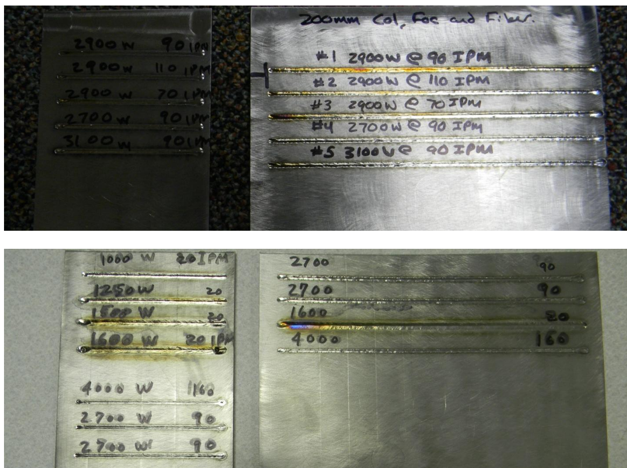
Figure 22. Laser welds on PM Ti-6Al-4V plate and extrusion samples.
