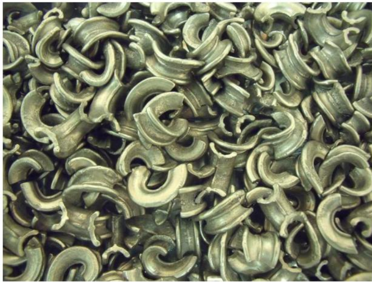
Figure 18. Cambridge process titanium from Metalysis Ltd, Rotherham, UK
