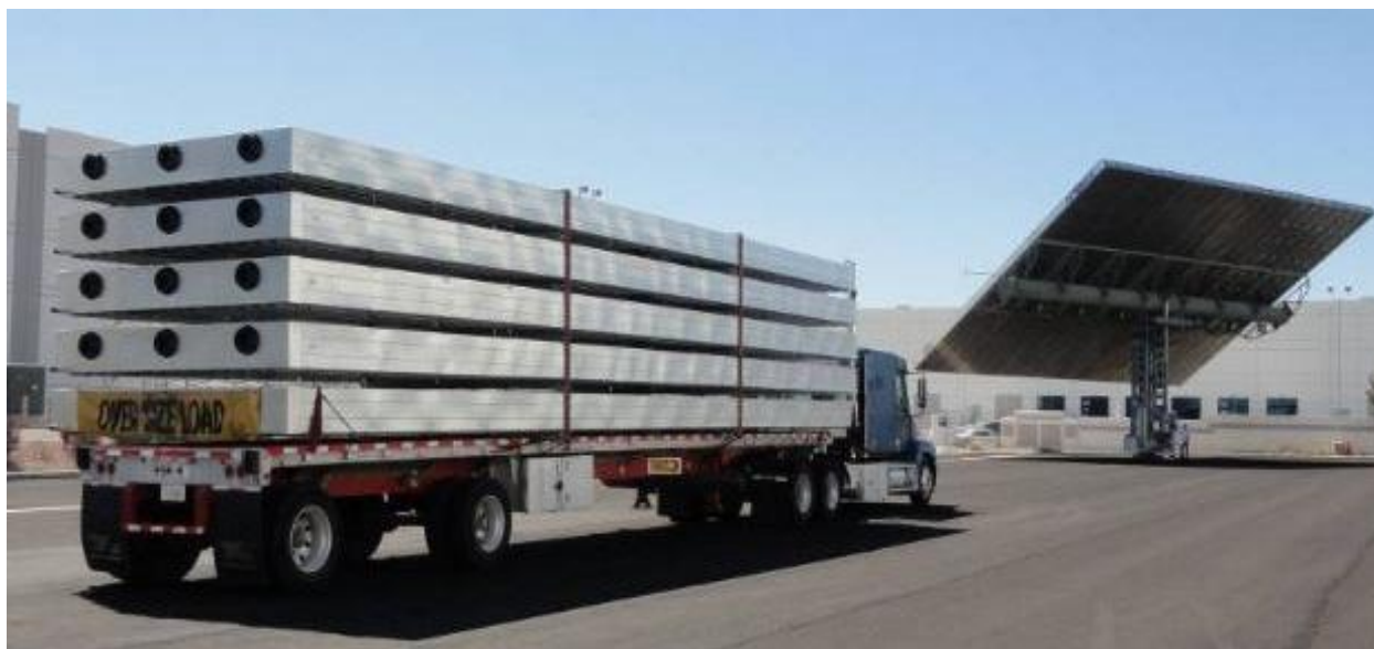
Figure 7-4: By shortening the height of the MegaModule's central welded structure, the Series-7700 MegaModules can be stacked 5-high on a trailer, without violating DOT truck-height restrictions.
