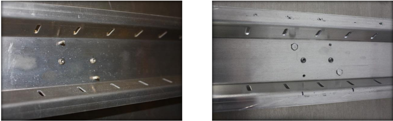
Figure 5-2. Alternative cooling fin fasteners: simple fastener (left), clinch (right).
