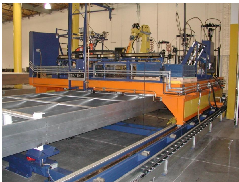
Figure 7-5. Lens alignment & installation robot.
