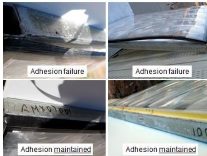
Figure 4-1: IEC 62108 testing of fast-cure adhesives for lens attachment.
