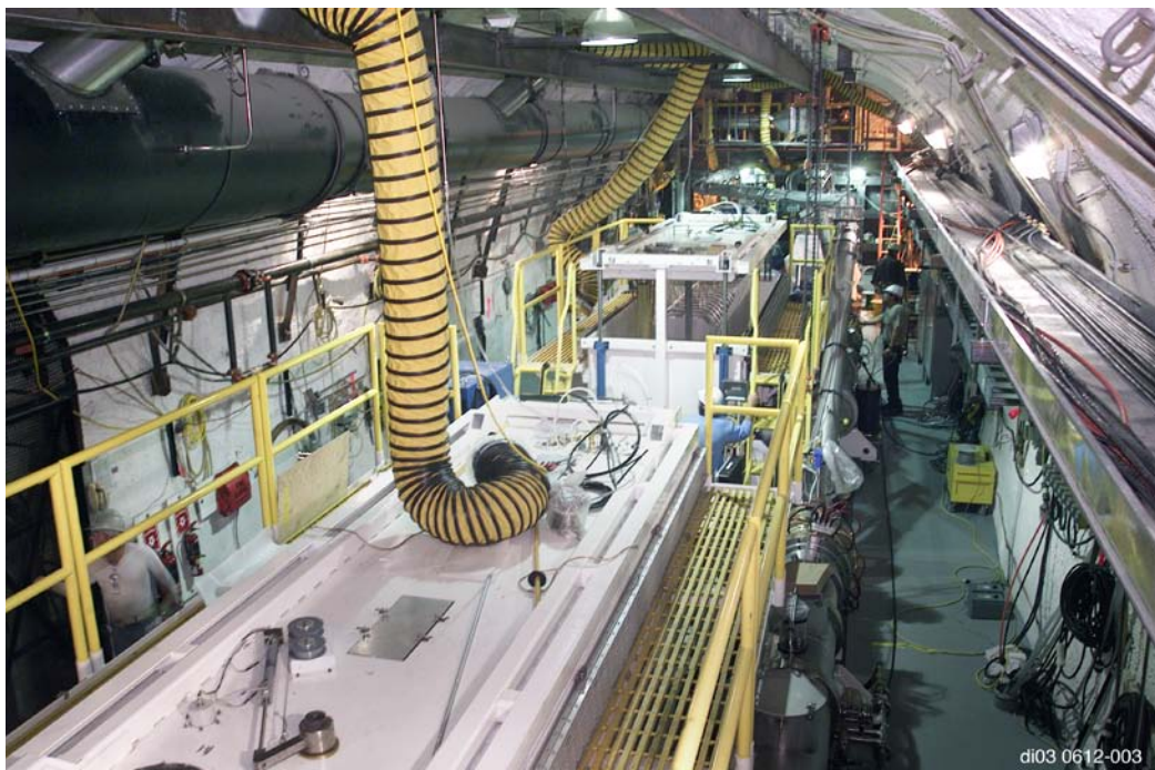
Figure 3. Cygnus 1 Marx Generator in the background (with lid raised), and Cygnus 2 Marx Generator in the foreground.
