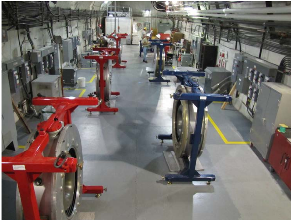
Figure 7. All six Cygnus IVA Cells mounted on individual work stands in the 05 drift awaiting refurbishment. Cygnus 1 cells are on red stands, and Cygnus 2 cells are on blue stands.
