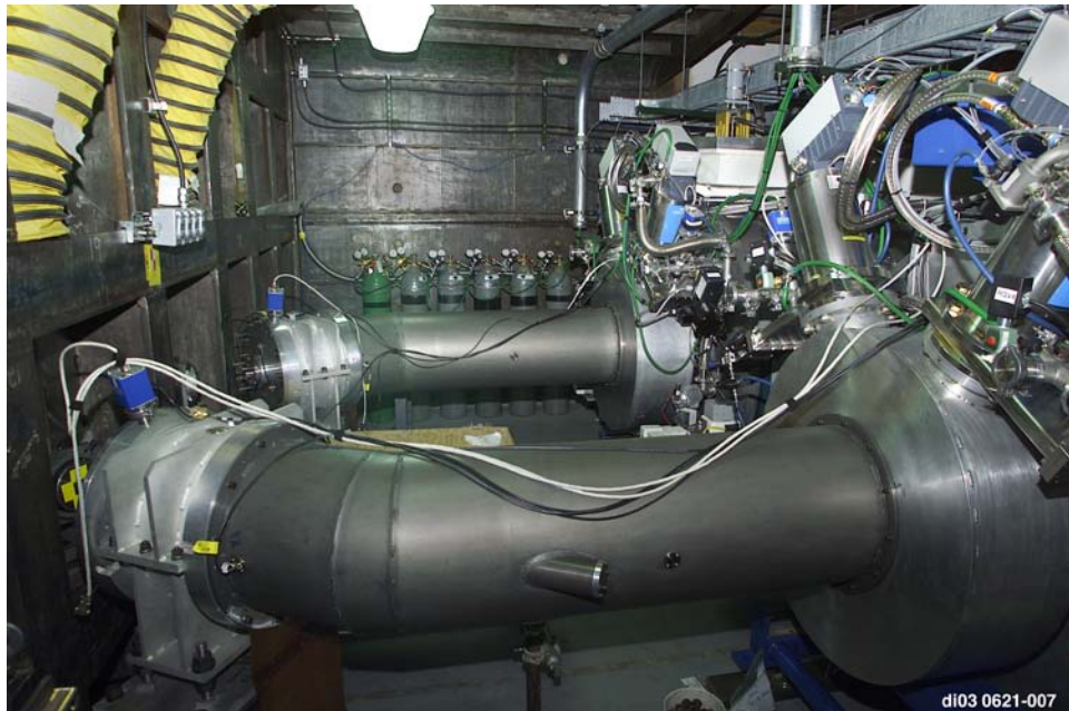
Figure 5. Cygnus 1 X-ray Diode (background, left), and Cygnus 2 X-ray Diode (foreground, left), with the barrier on the far left.
