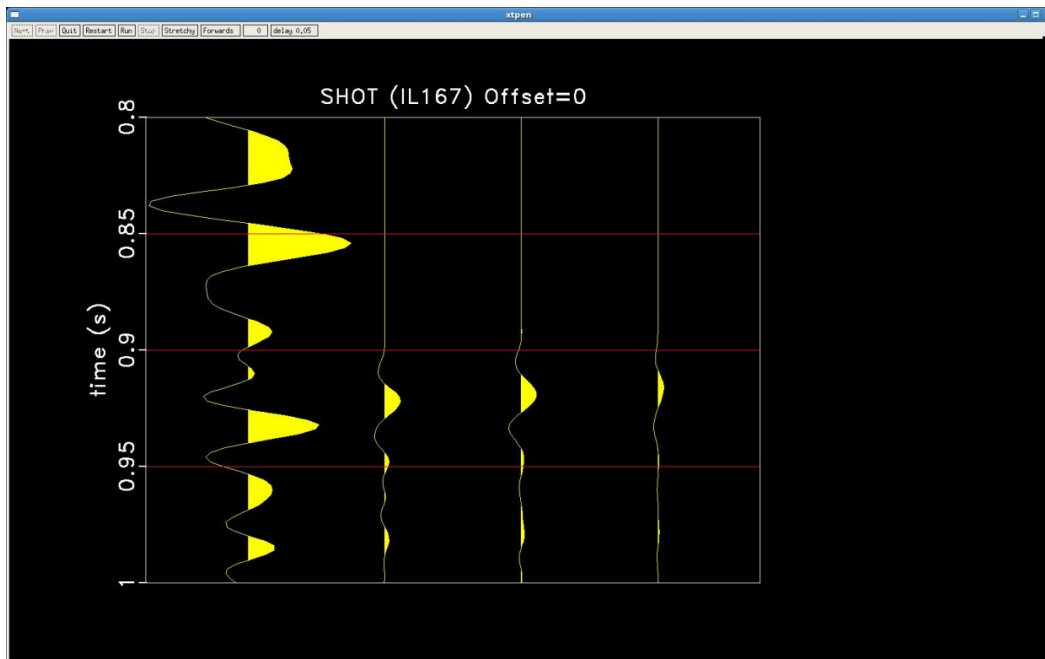
Figure 64: Comparison between the differences of the three injected models (CO2, 2040 and 3010) and the Baseline model. The first section shows the seismogram computed using the Baseline model. The second, third and fourth sections show the result of subtracting the seismograms computed using models CO2, 2040 and 3010 (respectively) from the Baseline seismogram in first section. Only the zero-offset seismogram is shown for all 4 sections.
