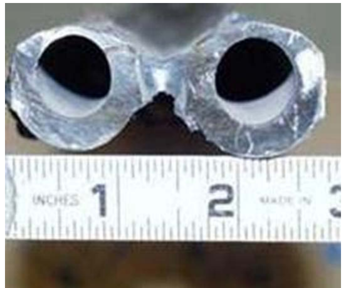
Figure 1-1 Photographs of waterwall and a cross section of tubes showing the extent of corrosion and wall-thickness wastage.
