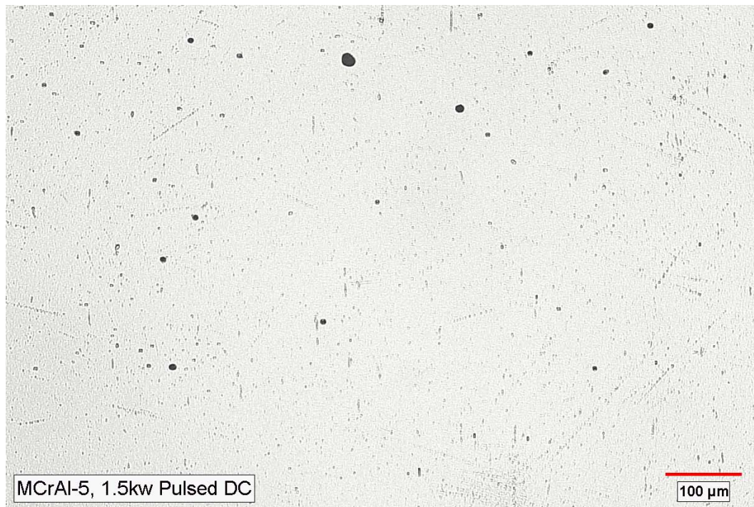
Figure 4-16 Optical micrographs of the pulse DC coated samples (top view) using 1.5 kW power to the Al target.
