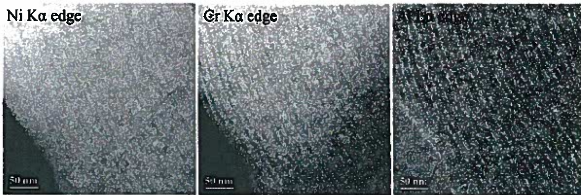
Fig. 19 Elemental mapping of the Ni-20Cr-3Al coating using Ni, Cr and Al ionization edges. It becomes clear from these images that the thin bands are Al-rich and that the thick bands are Ni-Cr-rich.
