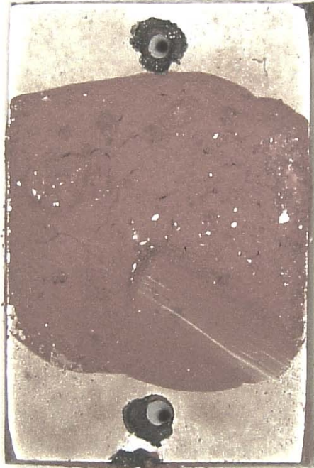
Coated H160 Al, Haynes, Eastern Ash, 816C, 500 hrs
