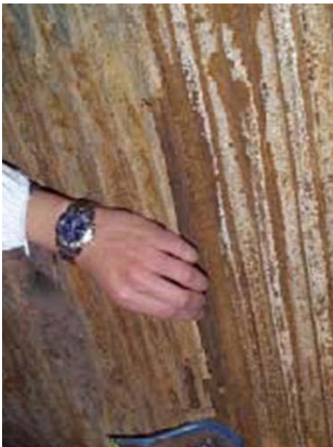
Figure 1-1 Photographs of waterwall and a cross section of tubes showing the extent of corrosion and wall-thickness wastage.
