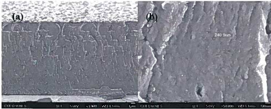
Figure 3. (a) Cross-sectional SEM micrographs showing the architecture of the CSM-3 coating; (b) superlattice structure with \Lambda=24 nm observed in the MCrAl layers.
