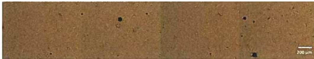
Figure 3. OM images of the thick SW3-MCrAl coatings deposited by PMS taken at four different locations on the as-deposited coating surface (including the worst surface defects observed on the coating surface).
