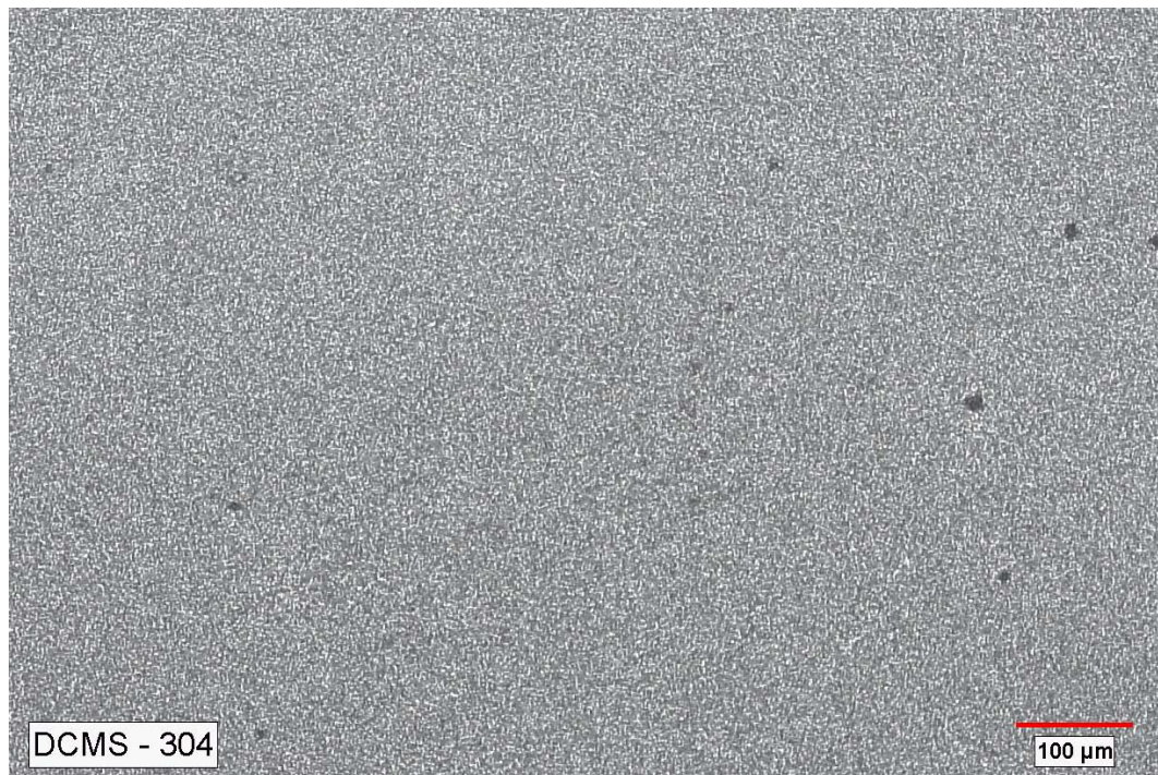
Figure 4-22 Optical micrographs of pulse DC coating (top view) on a) Haynes 230 and b) 304 SS samples.
