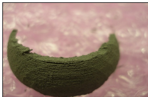
Figure 8. Layer fault due to interrupted printing
