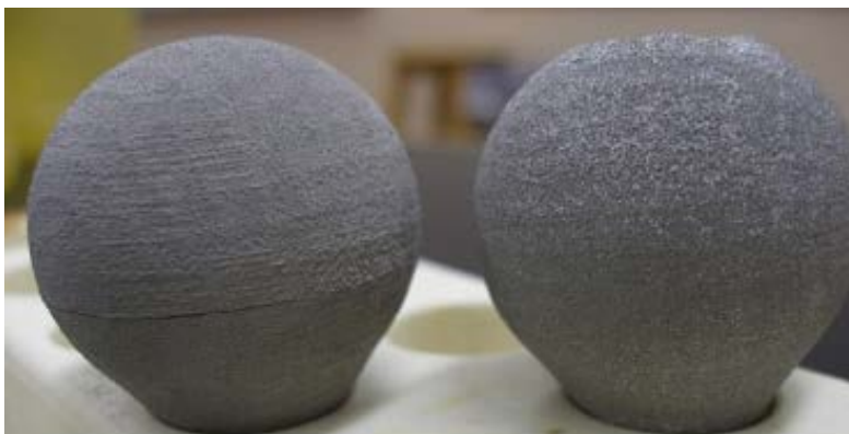
Figure 27. Cured substrate (left) and sintered substrate (right)
