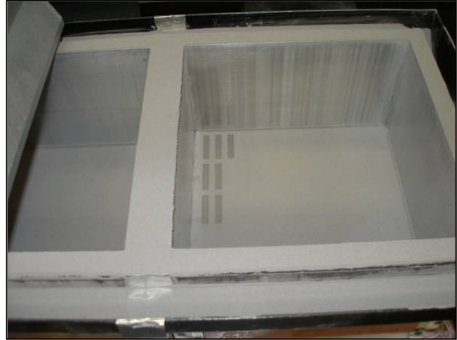
Figure 9. Feed box (left) and build box (right) at the end of a print job
