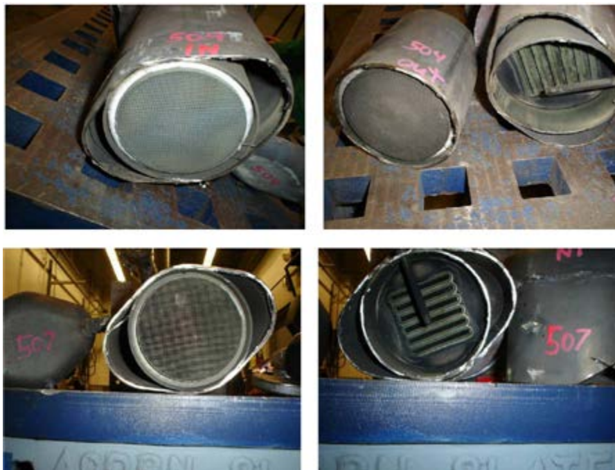
Figure 99. The ATR reactor vessels were cross-sectioned and examined.
