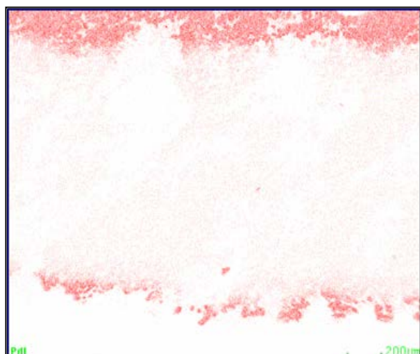
Figure 5. Palladium coating on substrate
