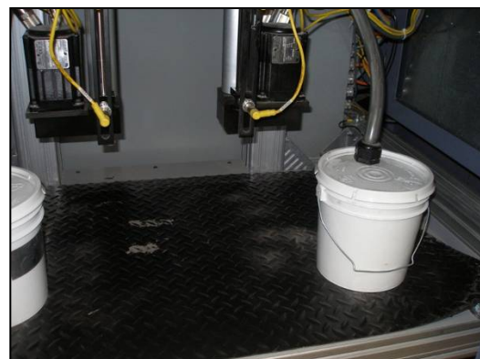
Figure 7. Titanium Dust in Lower Chamber
