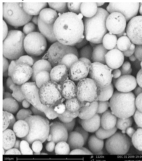
Figure 16. Sintering discoloration close up
