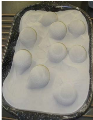
Figure 26. Photograph of nine bulb recovered from print job.
