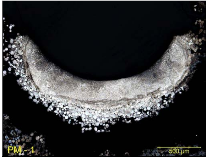
Figure 66. Welding on porous SS substrate (courtesy EWI)
