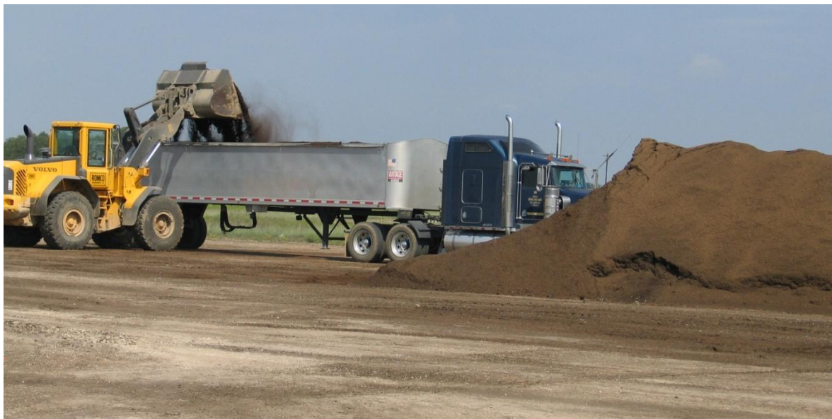
Figure D.6. Typical front-end loader utilized by CAFO facility to collect and load animal manure (DB or FB) for transport to a biofuel conversion facility.
