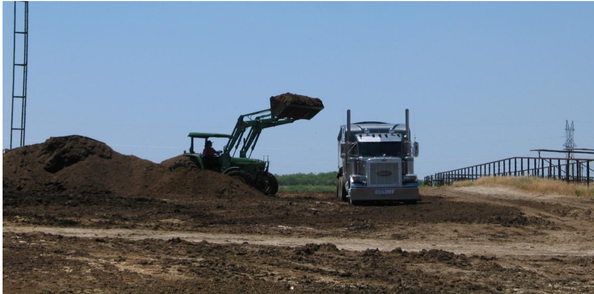
Figure D.7. An open-top truck with movable cover may be required for collection and transport of solid DB to large dairy facilities, or FB for cattle feedlots.
