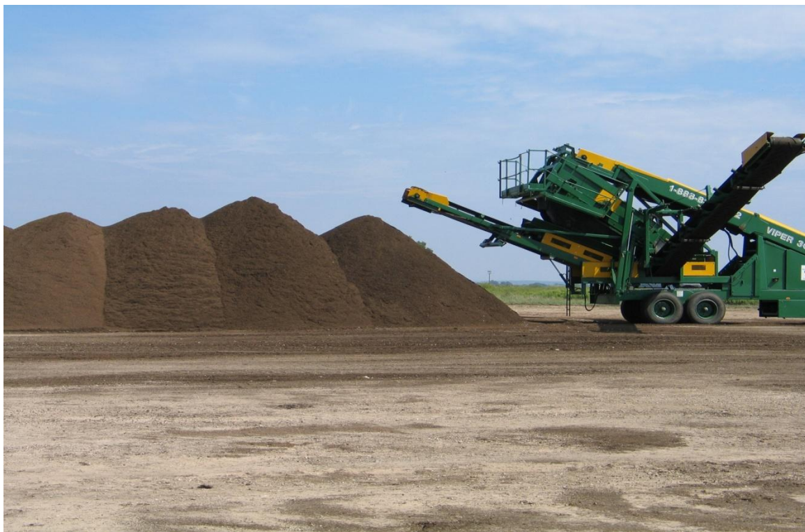
Figure D.8. A mechanical conveyor system can be used to collect animal manure (DB or FB), and transport to a centrally located collection and storage yard for subsequent conversion process (e.g. gasification).
