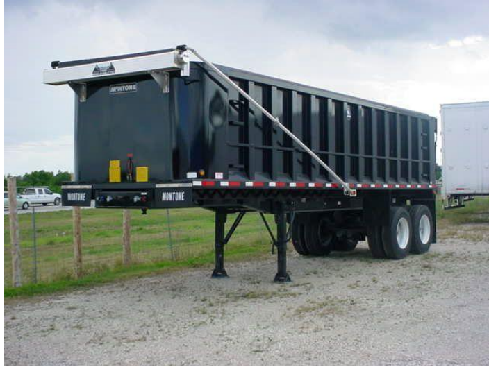
Figure 10.4.12 Montone 33.6 m 3 (44 yd 3 ) dump trailer (Montone Trailers, LLC., 2008)
