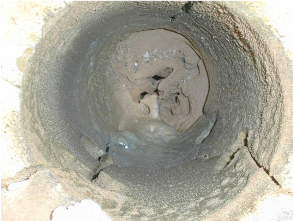
Figure 4.7.1. Top view of slag or melted ash deposits in furnace.
