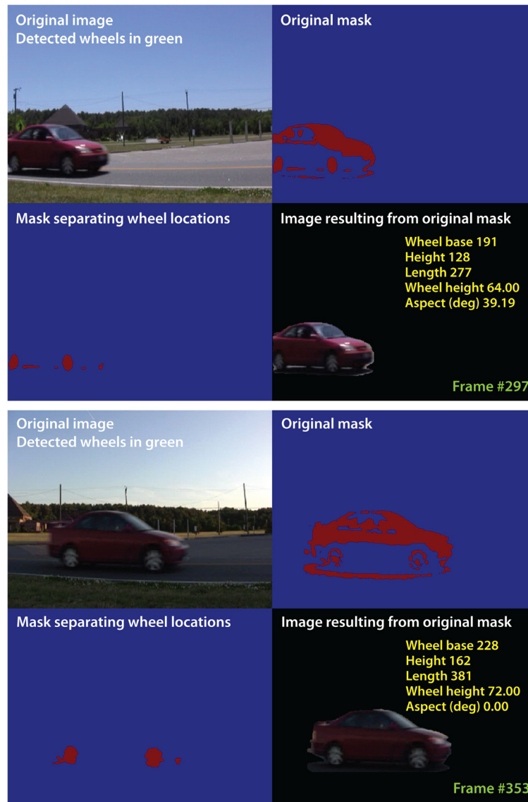
Figure 2. (top) Vehicle at 1:00 p.m. full sun; (bottom) images are for the same vehicle at 7:00 p.m. For each set of four images: (top left) original image with the wheel centroids in green; (top right) detected mask; (bottom left) wheel mask; (bottom right) extracted vehicle without the background. Dusk creates challenges for motion detection; atmospheric effects above tree lines and moving poles can cause false detects. The algorithms use a spatial filter to remove small areas of motion.
