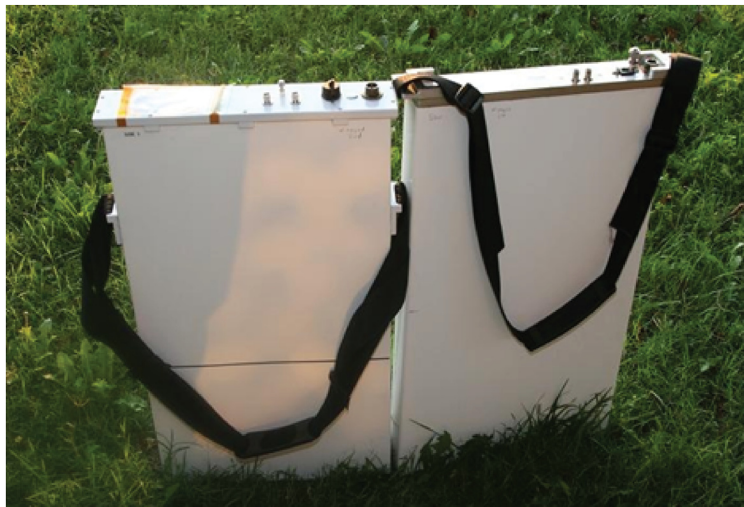
Figure 1. Two-panel NMC. The left panel has 100 straws and the right one has 60 straws. Each panel's external dimension is 70 \times 39 \times 6.25 cm and the combined weight is 29.4 kg (64.8 lb).
