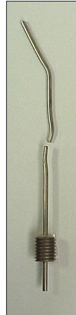
Figure 3 – Example photos of failures with complete fractures and single-wall fractures at third bend location.
