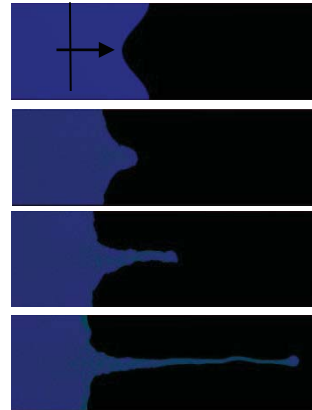
Fig. 1: MD calculations of jet-formation in Cu for 4 different groove geometries
