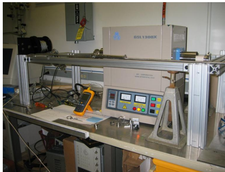
Figure 23: Lab setup for high-temperature fiber-optic strain sensor.
