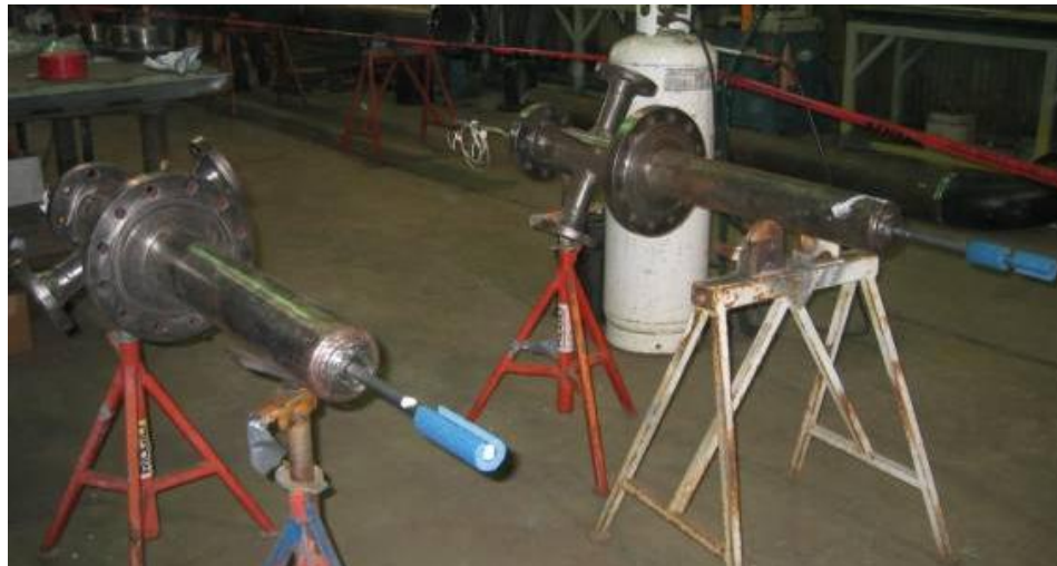
Figure 30: Soot-blower lances with temperature sensor package installed in TECO IGCC RSC.
