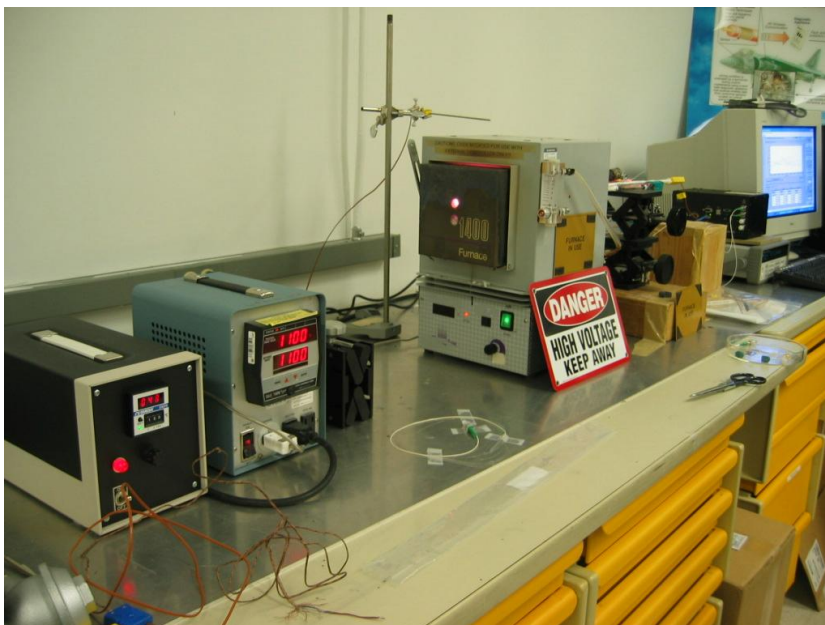
Figure 18: Lab setup for fiber optic temperature sensor short-term & long-term testing.
