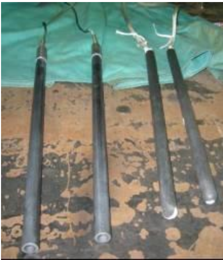
Figure 29: Four hexoloy radial temperature probes with integrated Type B TCs and FBG sensors (two probes on right) and single Type B TCs (two probes on left).
