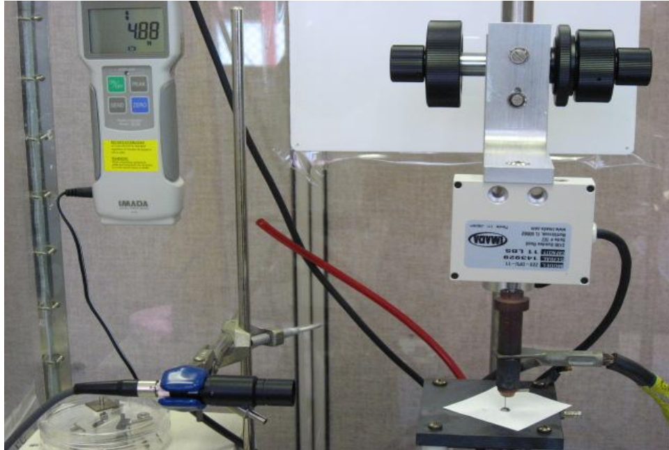
Figure A3. Anodic Bonder setup used to assemble Prototype 1 In-situ TEM chips.
