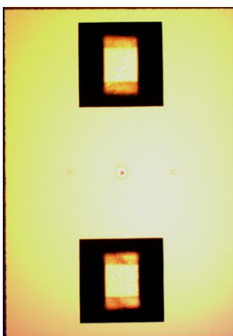
Figure A5. - Prototype 2 completed Top chip showing the ball lens facets and the TEM window at the center.
