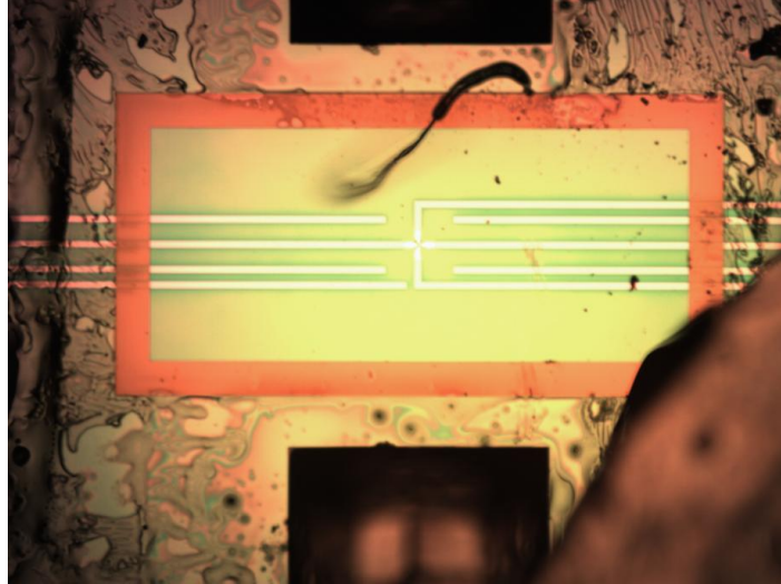
Figure A8. Disassembled bottom section of TEM chip prior to epoxy (EPOTEK 310) setting completely. No epoxy has seeped into the chamber but has wicked completely around the exterior of the ring.
